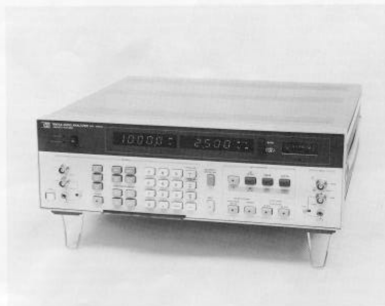
Fig. 1. Model 8903A Audio Analyzer makes the accurate measurements needed to characterize systems and signals in its frequency range of 20 Hz to 100 kHz. It has applications in general audio testing, transceiver testing, and automatic systems. Microprocessor control makes it automatic and easy to use.
