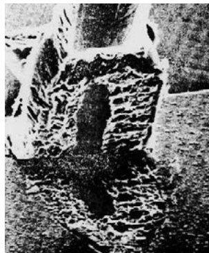
Figure 2 – After V.H. Winchell IEEE Proceedings 1978 – Low Frequency Weld Pattern
