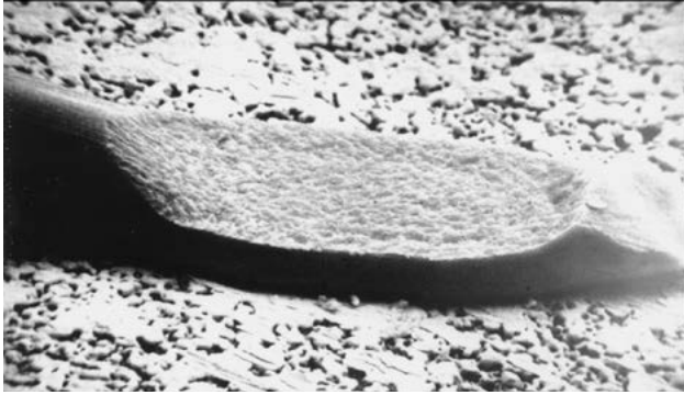
Figure 19 – Typical wedge lead bond. Tail length is minimal because the wire is terminated at this bond.
