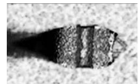
MaxiBond, no smash-out excellent 2nd bond termination
