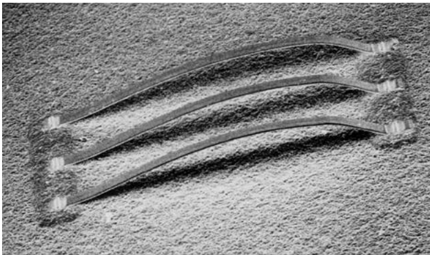
Figure 50 – Example of aluminum ribbon bonds. Note the cross groove impressions in the bonds.
