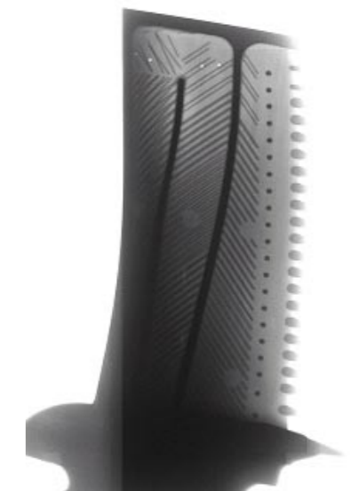
Radioscopy X-ray image of a turbine blade with flat panel detector
