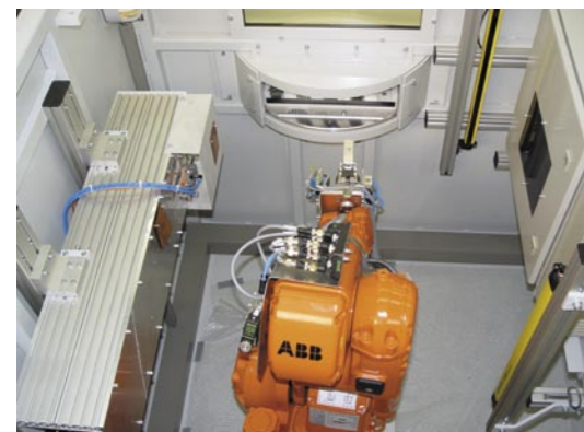
X-ray protection cabinet with ABB robot
