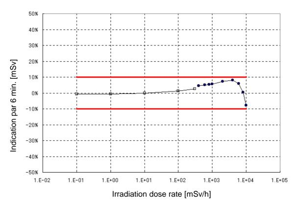
Open square is experimental data, black circle is simulated data using electric pulses.
