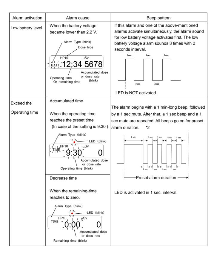
\*2 If the mode-switch is pressed in 3 seconds during preset alarm duration, the buzzer and LED are inactivated. (This Alarm-Stop-Function can switch ON and OFF using a setting device. Default setting is ON.)
