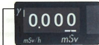
Indicates that the "**DOSE $\gamma$** " measures the Accumulated Dose of the Gamma-Rays in Measurement Mode.
