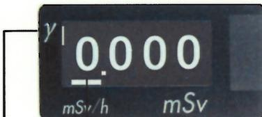
Indicates that the "**DOSE $\gamma$** " measures the Gamma-Ray Dose Rate in Measurement Mode.
