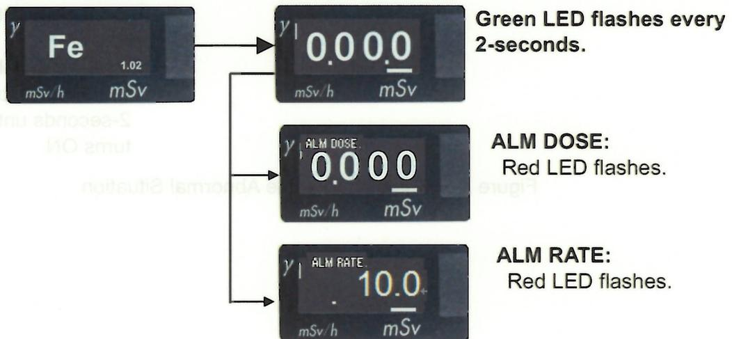
Figure 4-1 Display during Normal Situation
