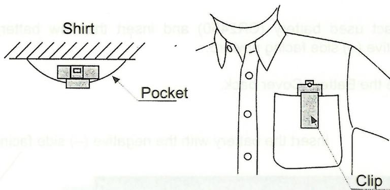
Figure 4-3 Inserting the "DOSE<sub>1</sub> - γ" into the Pocket
