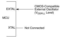
Figure 1-3. External Clock Connections (XCLKS = 1)
