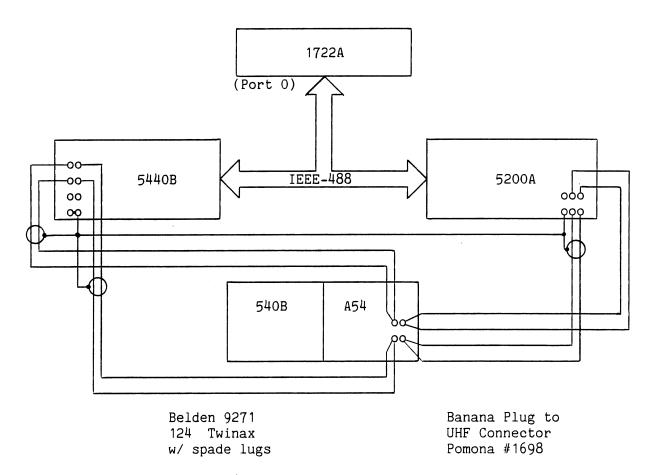
Figure 4-3. Equipment Setup, 5200A
