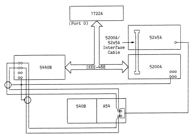
Figure 4-4. Equipment Setup, 5205A or 5215A
