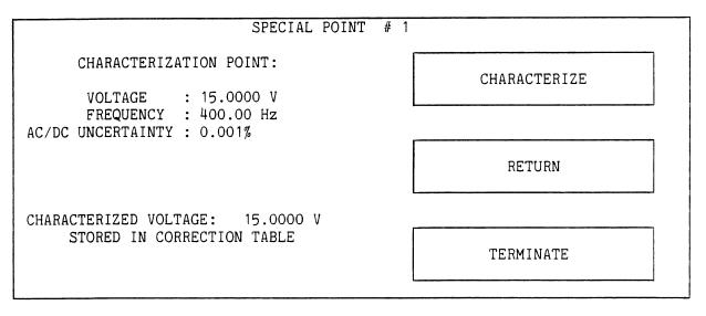
Figure 4-9. Special-Point Characterization Display
