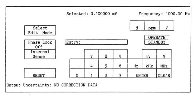
Figure 2-2. Data Entry Control Display
