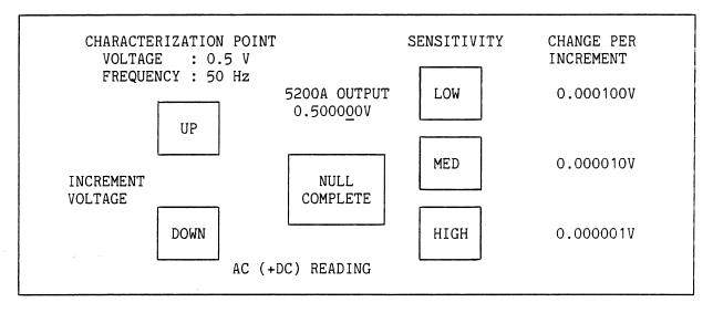
Figure 4-7. AC Null Control Display
