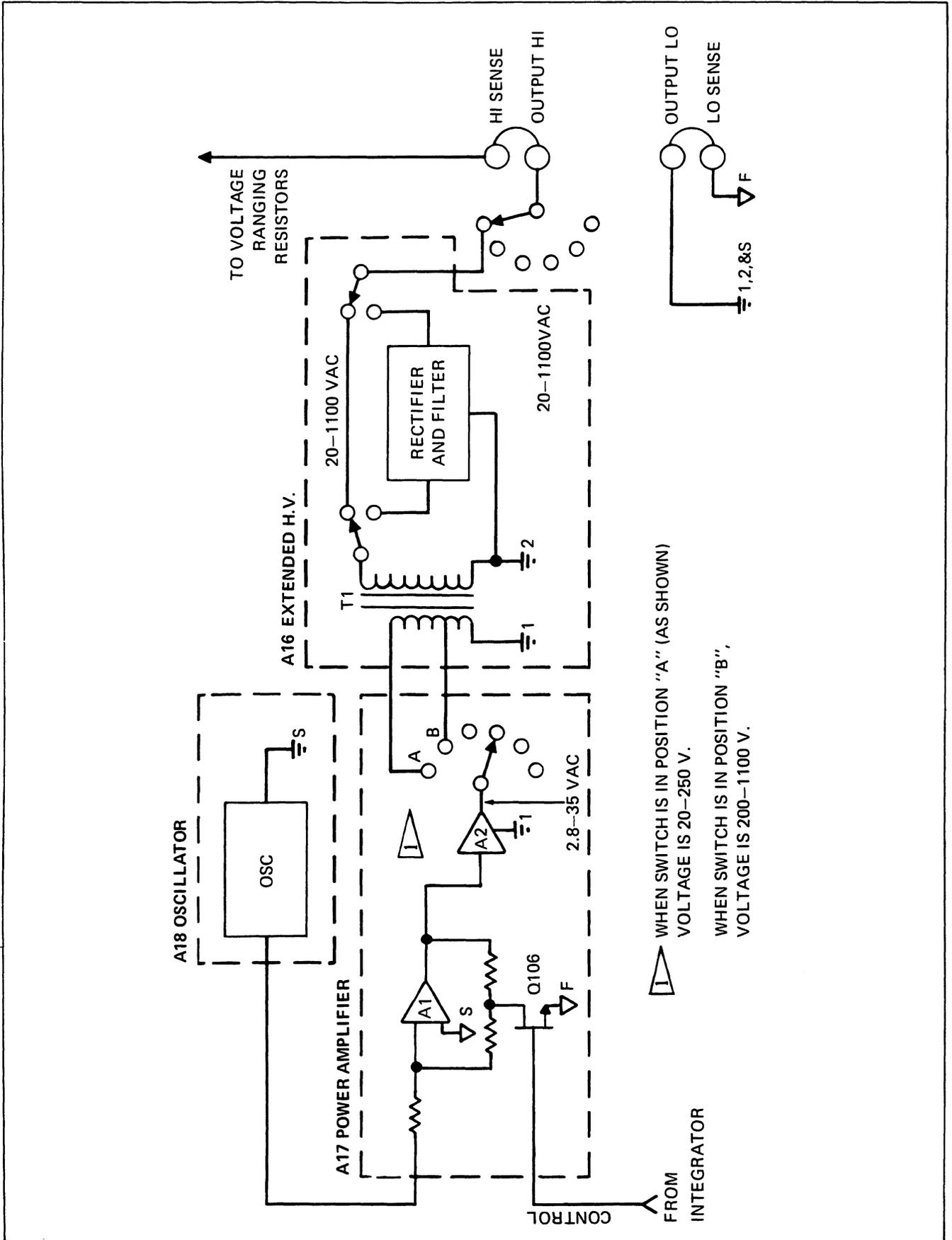
Figure 3-5. AC and DC Voltage, 20V and Higher
