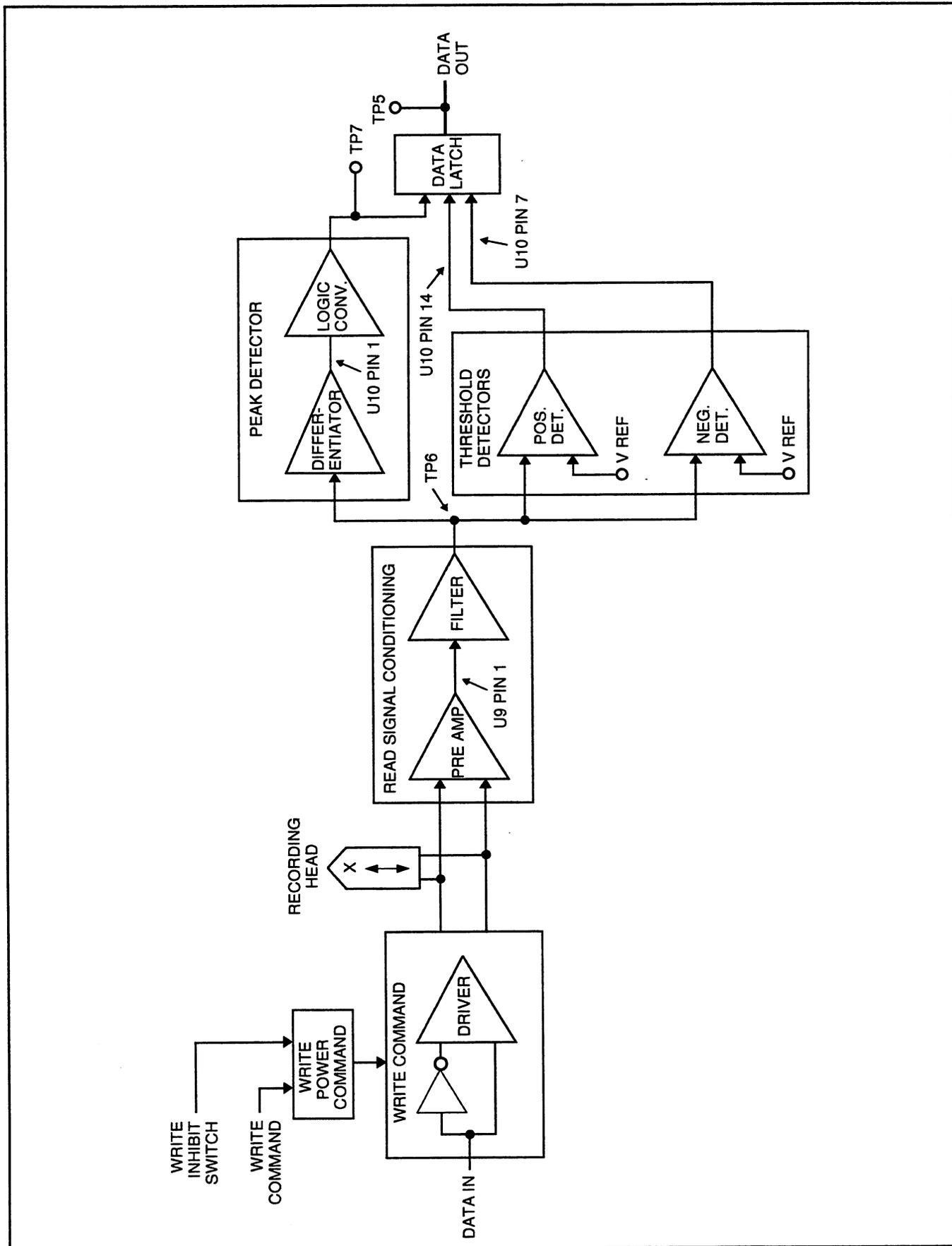
Figure 3-17. Read/Write Electronic Block Diagram with Accompanying Waveforms
