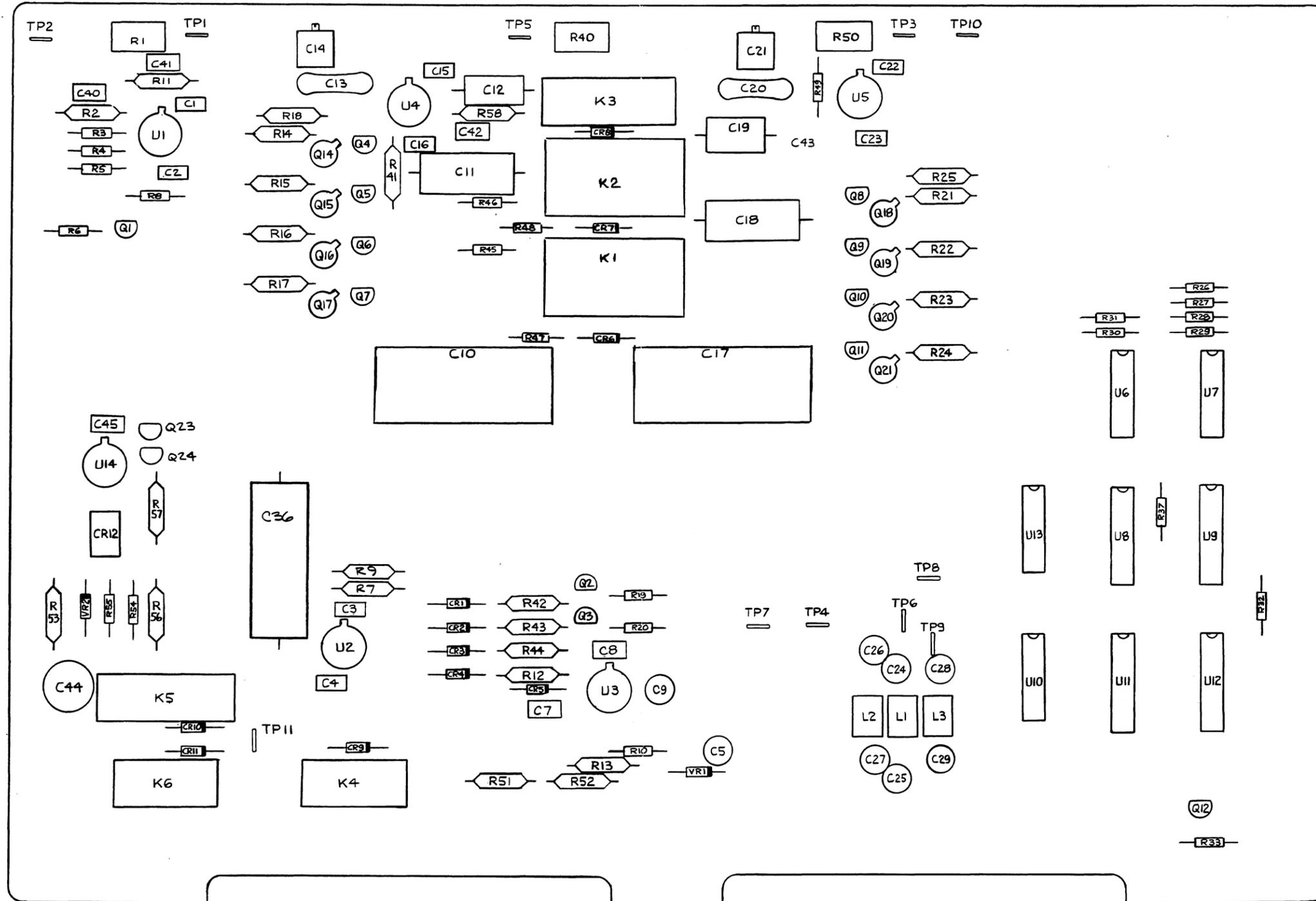
Figure 7-16. A18 Oscillator PCA
