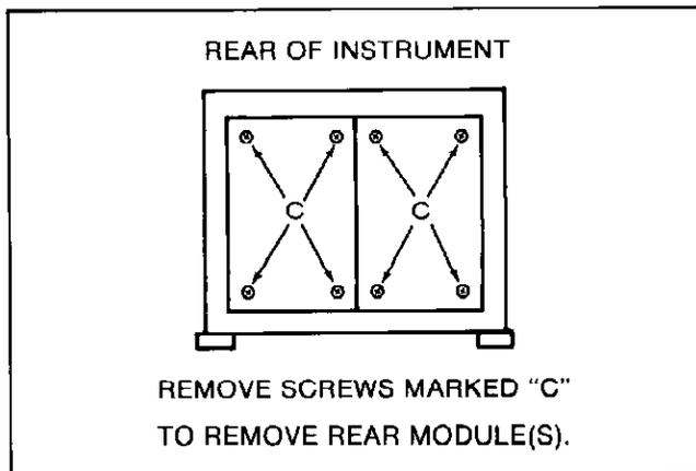
Figure 4-2. Rear Module Mounting Screw Locations
