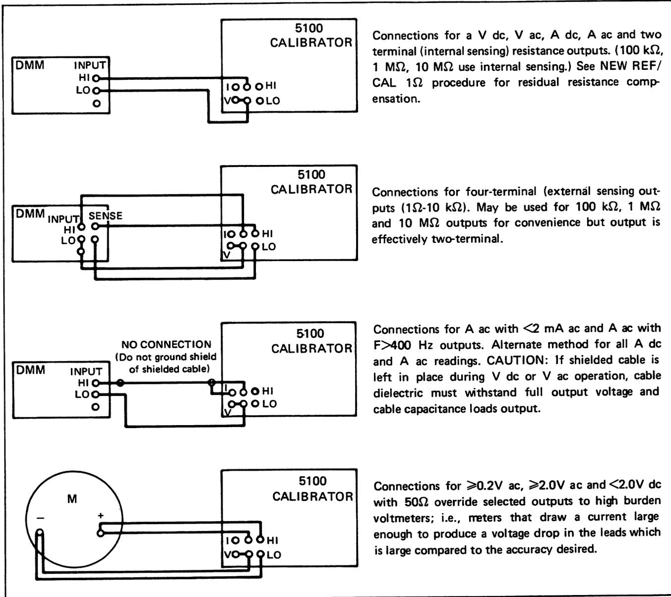
Figure 2-12. Meter Connections
