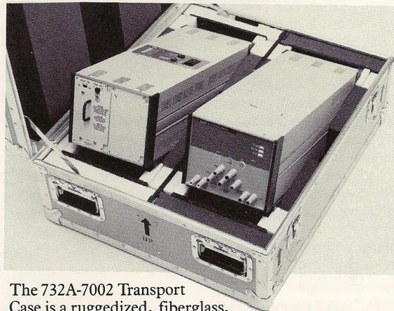
The 732A-7002 Transport Case is a ruggedized, fiberglass, foam-lined case capable of holding a 732A dc Reference Standard and a 732A-7003 Battery Charger, complete with up to four 732A-7005 Battery Packs. This extra battery capacity plus the heat-conserving insulation of the foam-lined case will extend the off-line operating time of the 732A to about 72 hours.
