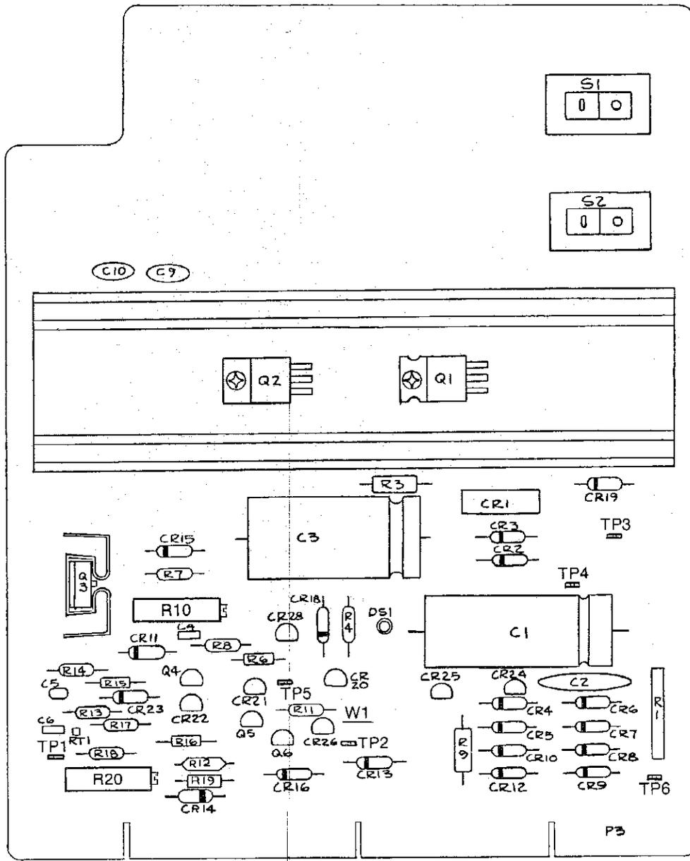
Figure 4-9. Battery Charger Test Points and Adjustments on A3 Pre-Regulator PCA
