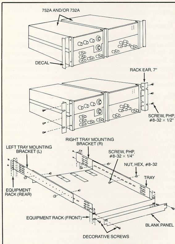
Installing the 732A-7004 rack tray kit.
