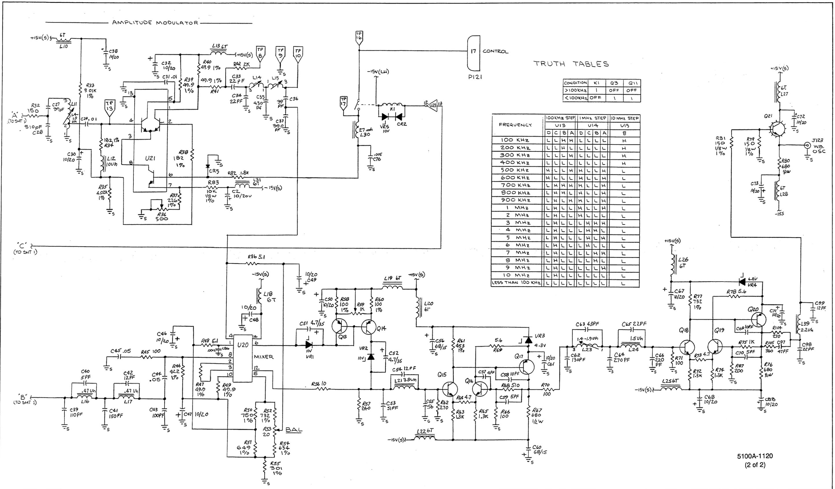
Figure 7-11. A13 Wideband Oscillator PCA (Option -03) (cont)
