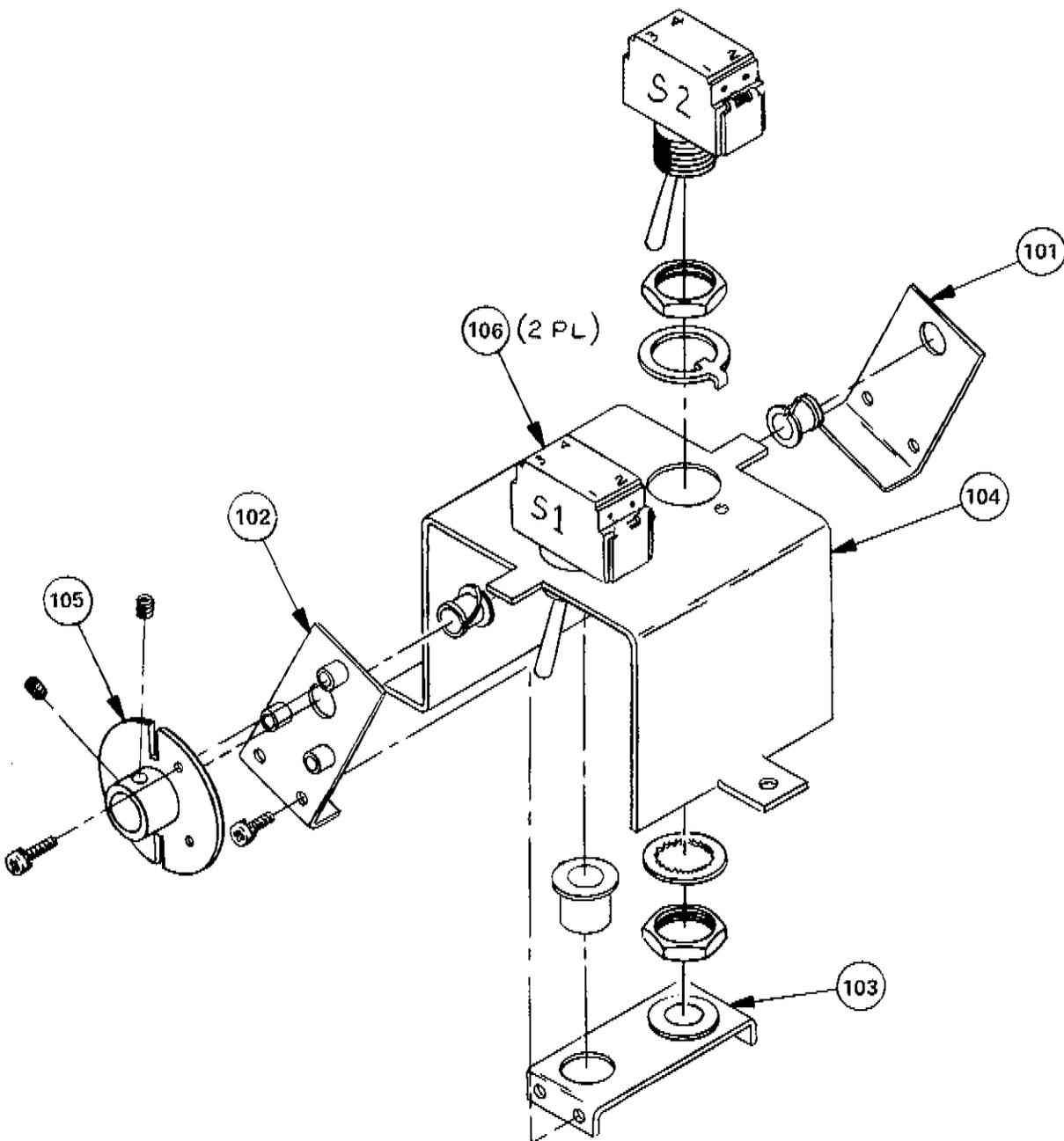
Figure 5-1. Power Switches View
