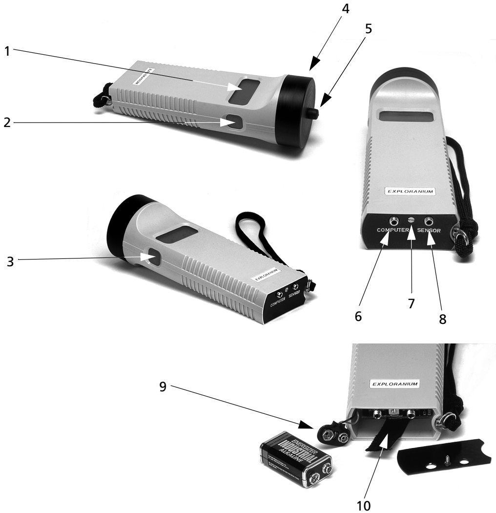
Figure 2 The controls and features of the KT-9.
