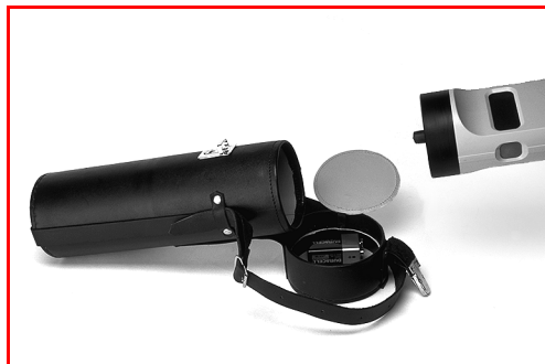
Figure 12 KT-9 orientation for storage. Note the compartment in the lid for storing a spare battery, studs and pins.
