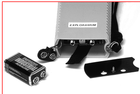
Figure 3 KT-9 battery compartment
