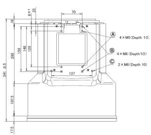
(A,B,C): Screw holes for fixing to apparatus
