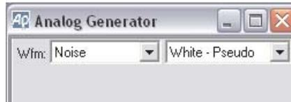
The **Noise: Pseudo** waveforms are analog-generated pseudo-random noise signals. The S2-BUR option is required to generate these waveforms. Three variations of the S2-BUR pseudo-random noise waveform are available:
