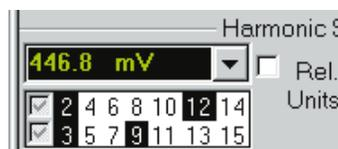
Figure 12-2 Distortion Order Control, Harmonic Sum Meters
