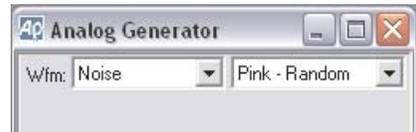
The **Noise: Random** waveforms are analog-generated true random noise signals. The S2-BUR option is required to generate these waveforms. Three variations of the S2-BUR random noise waveform are available:
