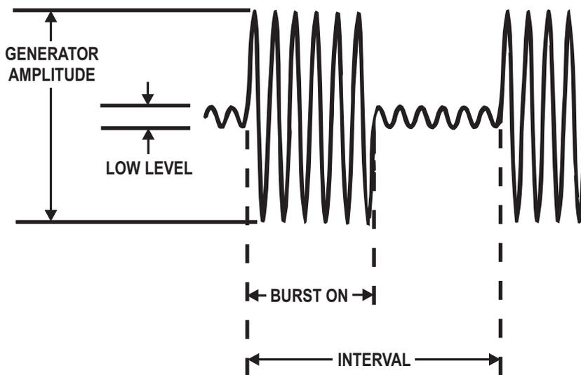
Figure 4-5 Tone Burst Definitions, Burst Normal Waveform
