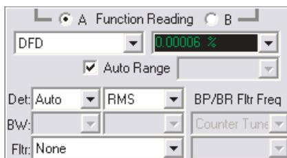
The **DFD** (difference frequency distortion) IMD measurement is made in the same way as a CCIF measurement, differing only by amplitude calibration. DFD results are expressed as values 6.02 dB lower than CCIF.
