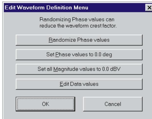
Figure 16-8 Edit Waveform Definition Menu, Utilities Multitone Creation
