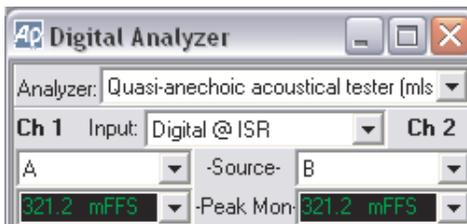
The two **Peak Mon** meters on the MLS panel continuously display the peak amplitude of the digital signal as it is presented to the MLS Analyzer. Only digital domain units (**FFS**, **dBFS**, **%FS**, or **bits**) are available for these meters.
