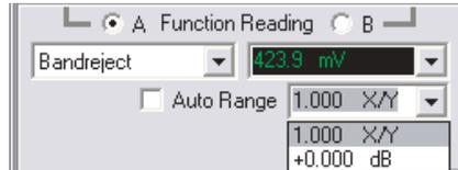
Like the Level meters, the Function meter has an amplitude ranging control, which is located lower on the Analog Analyzer panel beneath the Function meter reading field. See page 130 for a discussion of fixed and automatic ranging.
