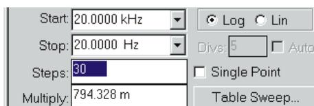
Figure 20-5 Log Sweep; Resolution Value is Constant “Multiply” Value
