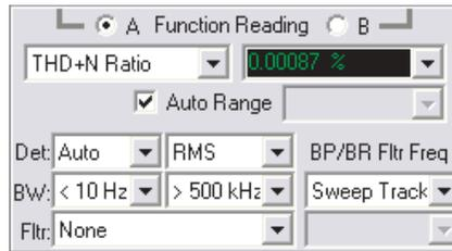
In the **THD+N Ratio** function, the selected channel signal is filtered in the same way as the **THD+N Ampl** function, above. The difference is in the expression of the result.
