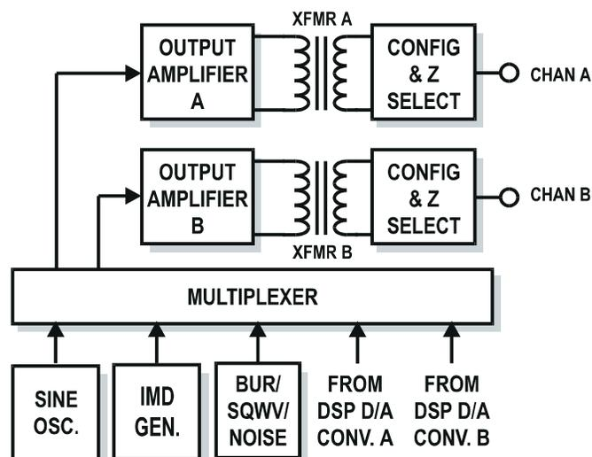
Figure 4-14 System Two Analog Generator, Simplified Block Diagram
