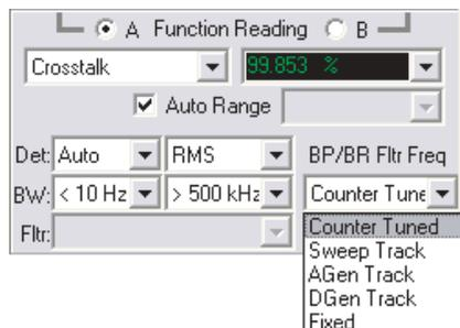
In the **Crosstalk** function, detector, reading rate and high-pass, low-pass and option filter selections are enabled.
