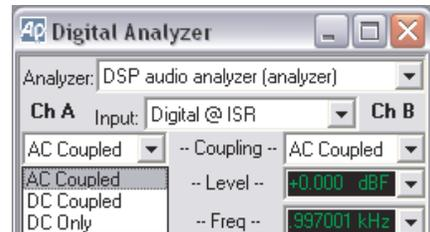
The Coupling selections in the DSP Audio Analyzer affect only the Level meter readings. The Function tools always have a high-pass filter in the measurement path, and therefore are always ac coupled. See the block diagram in Figure 178.
