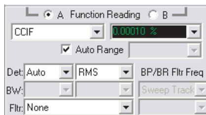
The Analog Analyzer **CCIF** function measures intermodulation distortion to the CCIF standard. A specific CCIF test signal comprised of two tones, F1 and F2, is applied to the DUT, and **CCIF** measures the amplitude of the difference product ( $F2 - F1$ ). This is recovered by first passing the signal through a 30 Hz high-pass filter and a 2.45 kHz low-pass filter, then applying a narrow bandpass filter that is automatically tuned to the difference frequency product.
