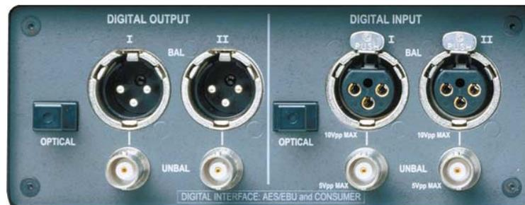
Figure 1-3 Digital Input/Output (Lower Left) Connector Panel
