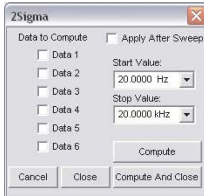
**Compute: 2-Sigma** is used with a series of wow and flutter measurements versus time (chart recorder style) when it is desired to have a single number representing the wow and flutter performance.
