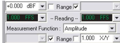
Most devices have an optimum amplitude operating range in which they exhibit their best performance. The 2700 series gives you the choice of automatic ranging (or *autoranging*) or a manually-set fixed maximum range.
