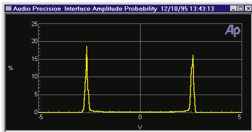
Figure 8-15 Probability vs Amplitude (5 V p-p Interface Signal)
