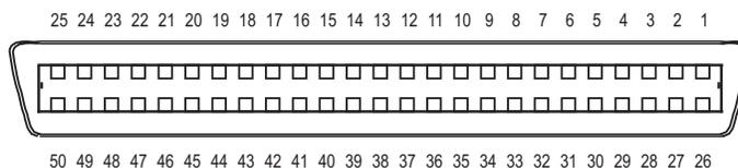
Figure 9-4 Parallel Input and Output Connectors
