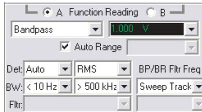
The **Bandpass** function is a selective voltmeter (a function sometimes called a *wave analyzer*). The selected channel is passed through a four-pole 1/3-octave tunable bandpass filter before its amplitude is measured, to accomplish a frequency-selective amplitude measurement. The bandpass filter center frequency can be set in the range between 10 Hz and approximately 204 kHz. The center frequency may be fixed, or may track one of several parameters; see **BP/BR Filter Tuning** on page 149.
