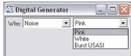
The 2700 series Digital Generator offers three DSP-generated pseudo-random noise signal selections: **White**, **Pink** and **Burst USASI**. The noise waveform amplitudes are calibrated in peak equivalent sine wave terms. See **Amplitude Control and Units** on page 101.
