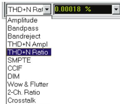
Figure 5-6 Function Reading Meter Function Selection List
