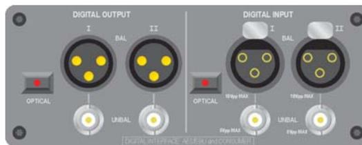
Figure 7. SYS-2722 main Digital Output and Digital Input.
