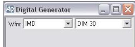
DIM is an acronym for *dynamic intermodulation*; another term for this IMD test is TIM, or *transient intermodulation*. Like the Analog Generator DIM waveform selections (page 83), the three **IMD: DIM** choices linearly combine a square wave near 3 kHz with a higher-frequency sine wave. The peak-to-peak amplitude ratio of the square wave to the sine wave is 4:1.
