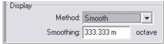
MLS octave smoothing is a Display Method that shows MLS frequency domain results as modified by a smoothing algorithm. Smoothing only operates on frequency-domain displays.
