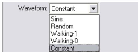
The Digital Data Analyzer can perform bit-error measurements on five different digital domain stimulus waveforms, chosen in the Waveform selection field. Each waveform has a specific testing application.
