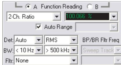
The **2-Ch Ratio** function displays the ratio of the Function meter reading for the selected channel to the Level meter reading for the opposite channel.
