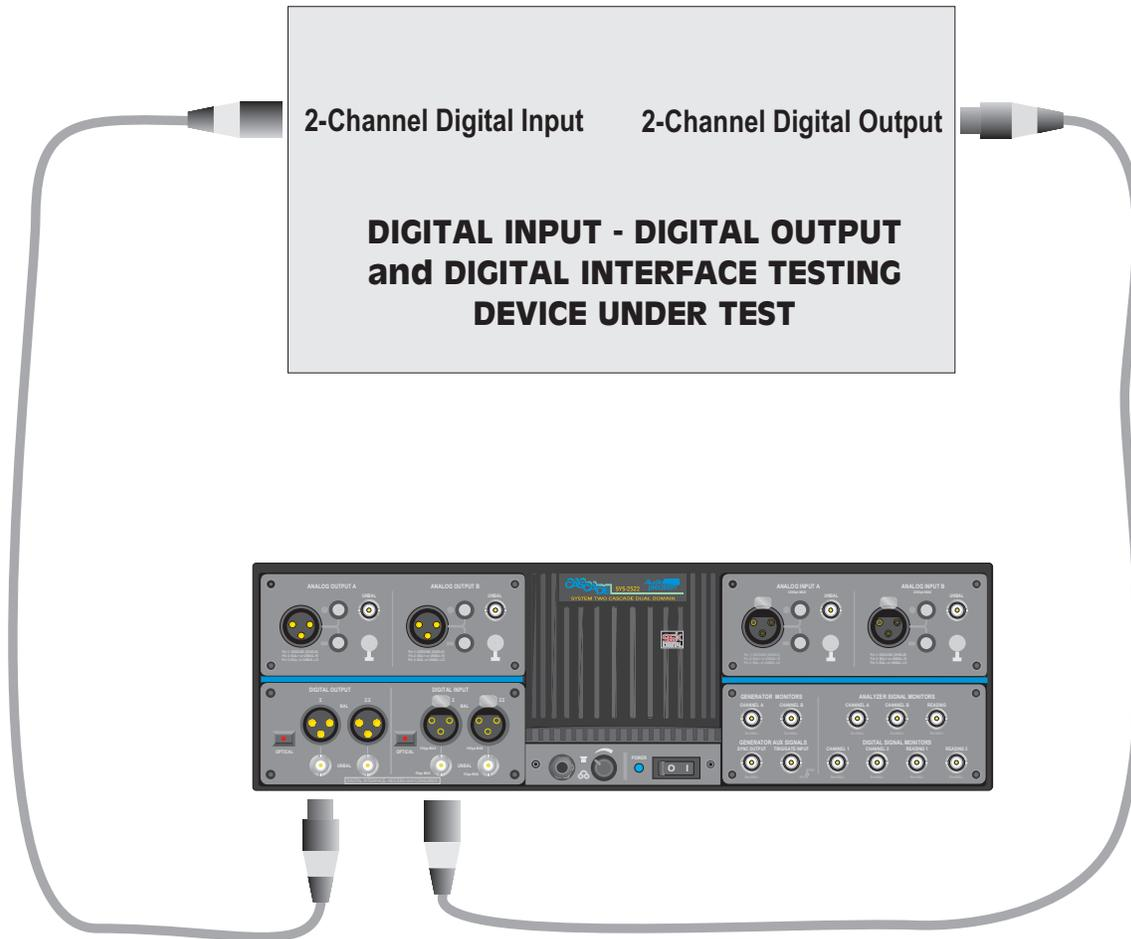
A System Two Cascade Dual Domain (SYS-2522) series instrument is required for these tests. A standard installation places System Two Cascade digital interface tests in the **C:\APWIN\S2CASCADE\DIOANALYZER** subdirectory.
