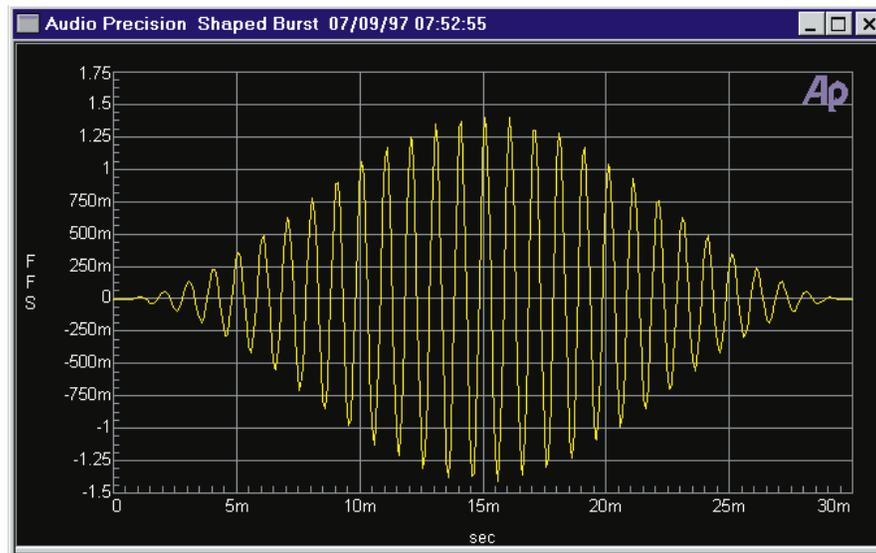
Figure 10-4 Shaped Burst of 1 kHz Frequency, 30 Cycles Duration
