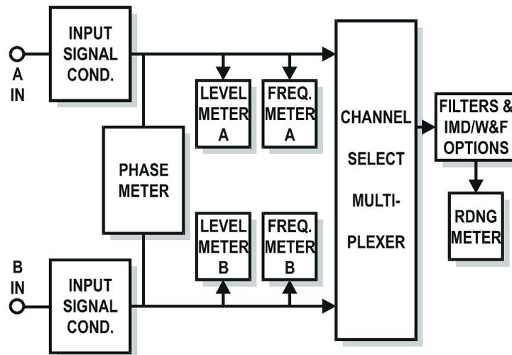
Figure 5-17 System Two Analog Analyzer, Simplified Block Diagram
