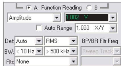
In the **THD+N Ampl** (amplitude) function, the selected channel signal is passed through a tunable bandreject (notch) filter in order to reject the fundamental component of an applied single sine wave test signal before the amplitude of the remaining distortion and noise components is measured and displayed. The filter is continuously adjusted for maximum rejection of the highest-amplitude frequency component of the signal.
