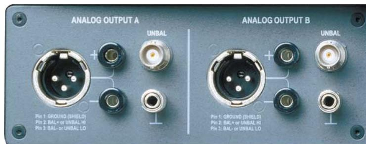
Figure 1-2 Analog Generator (Upper Left) Output Connector Panel
