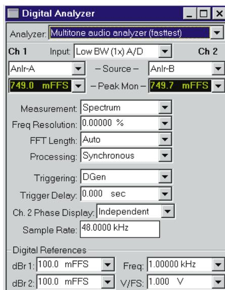
Figure 16-1 Multitone Audio Analyzer (FASTTEST), large version
