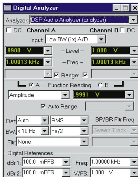
Figure 11-2 DSP Audio Analyzer Panel, Large Form
