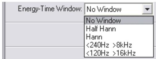
When **Energy-Time** is selected as the time domain display, a frequency window can be selected in the Energy-Time Window field to reduce aliasing behavior in the transformations applied.
