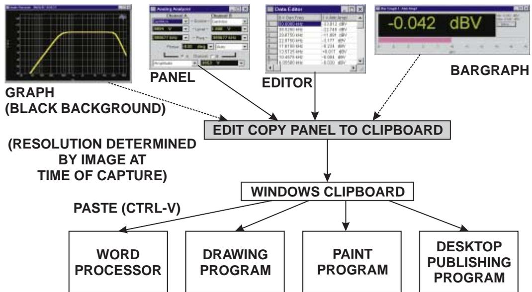
Figure 21-15 Schematic Representation of Various Hardcopy Techniques
