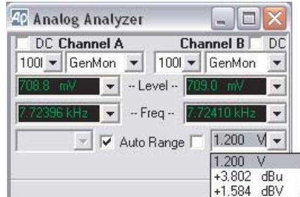
Practical devices have an optimum amplitude operating range in which they exhibit their best performance. This is true for amplifiers, for measurement instruments and for the ADC circuits used in the 2700 series for conversion to the digital domain. The 2700 series uses selectable attenuators and amplifiers to bring a wide range of input signals to the optimum amplitude for the measurement detectors.
