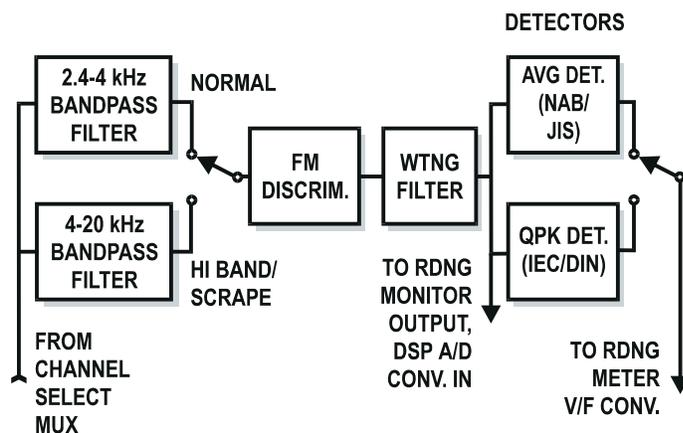
Figure 5-8 Wow and Flutter Analyzer Option, Simplified Diagram
