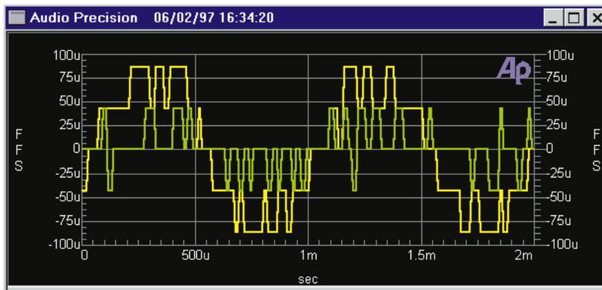
Figure 15-9 -85 dBFS and -100 dBFS 16-bit sine wave signals, normal dither, no averaging.
