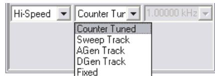
The Harmonic Distortion Analyzer must identify the fundamental frequency that you have selected for your measurement. The amplitude of the fundamental component is used as the basis of the Ratio measurements, and the precise
