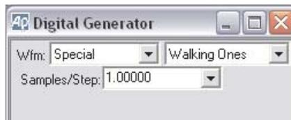
**Walking Ones** is a signal in which only one bit is at logical “one” at any moment, with the others all at logical “zero.” The position of the bit which is at logical “one” is stepped through the word from LSB to MSB repeatedly, at a rate controlled by the **Samples/Step** field.
