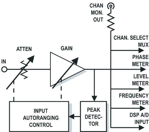
Figure 5-18 System Two Analog Analyzer, Simplified Diagram of Input Channel. Channels A & B Are Identical and Independent
