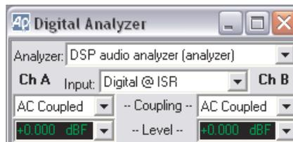
Two Level meters are located near the top of the DSP Audio Analyzer panel, one for each input channel. The Level meters display the audio amplitude of the input signals. These meters are true rms meters, using a normal or a fast rms detector as selected in the right-hand Detector (Det) field lower on the panel. Level meters have selectable coupling, as discussed above.
