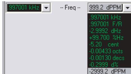
The frequency of the signals on the two channels are shown in the Freq meter fields, just below the Level meter readings. In documentation, the frequency meters are sometimes called frequency *counters*.
