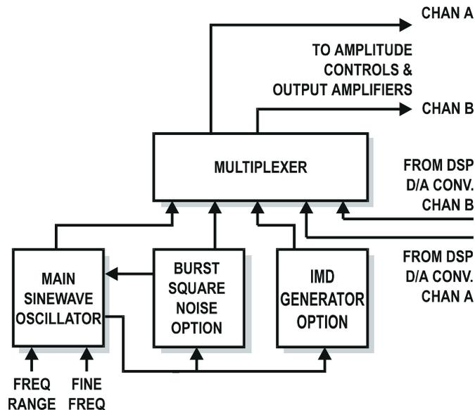
Figure 4-15 Oscillator Section, System Two Analog Generator
