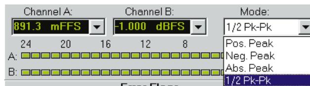
Figure 7-2 DIO Panel Peak Monitors and Mode Selection
