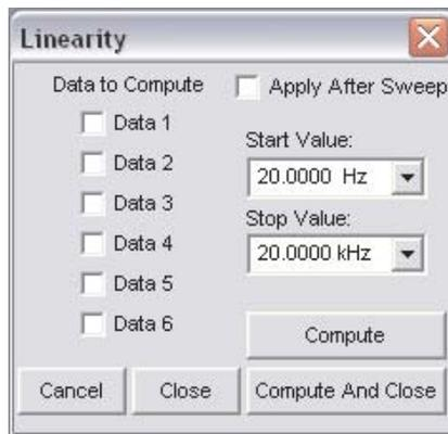
Typically, a DUT will have its greatest nonlinearity at the measurement extremes. To keep this atypical data from affecting the initial straight-line fitting, you can enter values in the **Start Value** and **Stop Value** fields to limit the range of data examined. These values only limit the straight-line computation; after the line is derived, every data point in the trace is subtracted from the line value.
