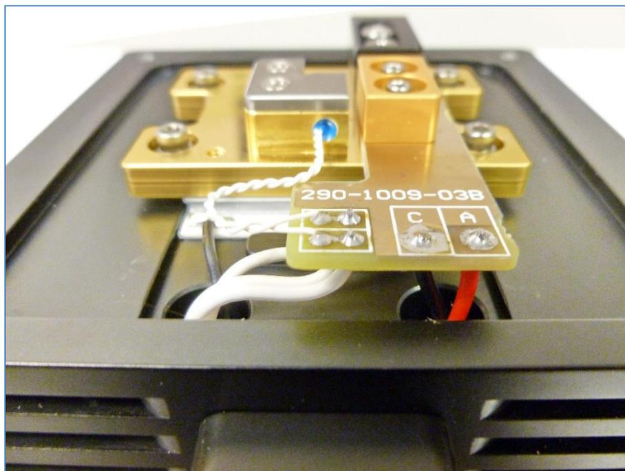
The process will be to disassemble the 290-1009-03 PCB from the cold plate, reverse the wires, then reassemble.
