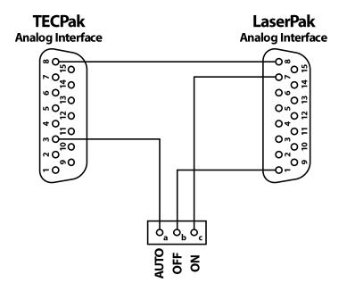
Use a three position switch (connect-open-connect) to connect switch terminals a+b in the AUTO position, terminals b+c in the ON position, and no connections in the OFF (middle) position. In this way, you will be able to control the laser manually, or operate it in automatic mode, based on the position of the switch.
