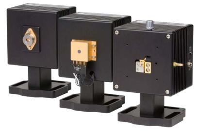
The 240 Series LaserMounts support C-Mount, HHL, and TO-3 devices for high performance and long term operation. All mounts feature solderless connections and an integrated fan for maximum thermal performance. Each fixture includes a removable pedestal, and is easily mounting to an optical table.
