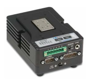
The 207 LaserMount offers dependable thermal control for the many LEDs and medium-powered fiber pigtailed lasers in the 5 to 10 watt range. With a user-configurable quick-disconnect electrical interface and broad device support, the 207 is an excellent choice.
