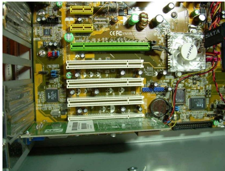
Figure 2. PCI-Express x1 (yellow), PCI-Express x8 (green), and Legacy PCI (white) Card Slots
