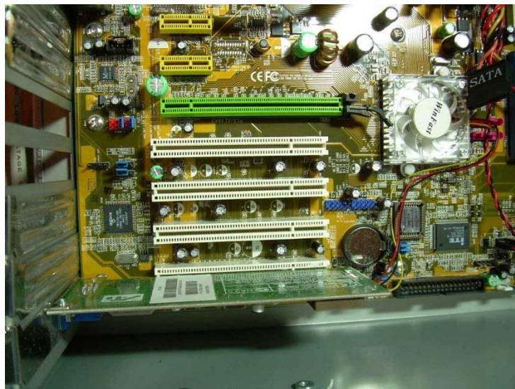
Figure 2. PCI-Express (green) and Legacy PCI (white) Card Slots
