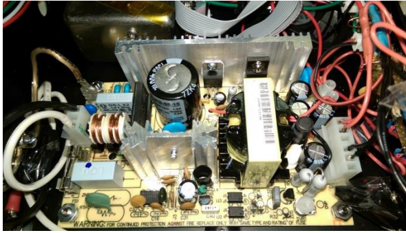
Figure 5.3: The 15V power supply. The regulator at the center of the heat sink is the L7805CV between the large electrolytic capacitor and the transformer. The leads for the associated capacitors pass through unused holes on the board.
