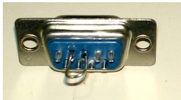
Figure 6.5: The loopback connector is a DB9 Female with a wire soldered between pin 2 and pin 3.
