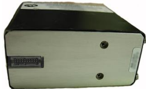
Figure 7.2: The FE-5650A Option 58 as viewed from the connector side. The AMP connector is on the left side and the two screws on the right side hold the front plate in place.
