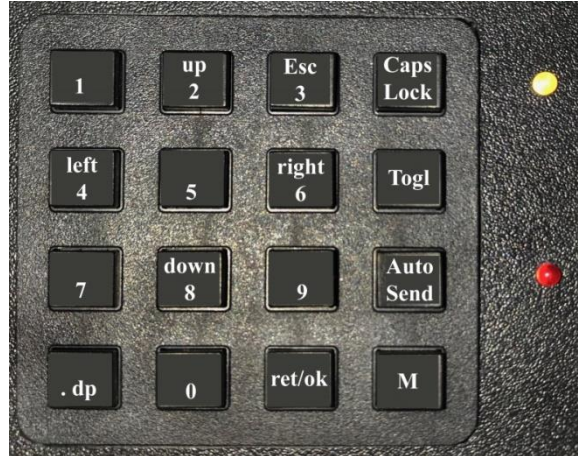
Figure 10.14: The keypad with labelled keys. The top LED indicates 'Caps Lock' and the bottom LED indicates 'Auto Send'.
