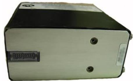
Figure 1.1: The FE-5650A Option 58 as viewed from the connector side. The unit is designed and manufactured by Frequency Electronics Inc. FEI.
