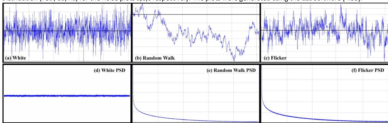
Figure 4.1: Panels a,b,c: White, random walk and flicker noise plotted versus time. Panels d,e,f show the Power Spectral Distribution (PSD, dB/Hz) for the noise plots a,b,c respectively. The plots were generated using the EZL Software [4.33].
