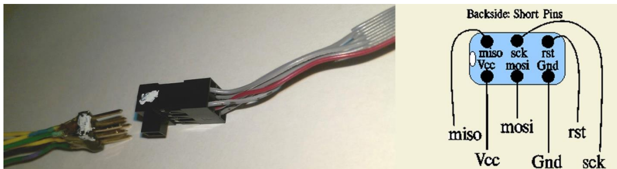
Figure 10.4: Left: The double row male header positioned next to the double row female receptacle for the Microchip-Atmel programmer. Right: View of the bottom side of the double row male connector (i.e., short pin side). The labels indicate the required connections to power and the microcontroller (Vcc = 5V and Gnd = ground = 0).
