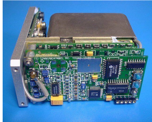
Figure 6.1: A view of the DDS board with J2 for the RS232 on the lower right side. And J1 with thin gray coax at upper left.
