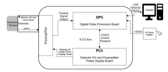
Figure 1. Connection Diagram. The detector can be FastSDD<sup>®</sup>, Si-PIN, or CdTe.
