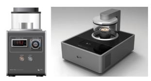
The Ion Sputter Coater allows for imaging of nonconductive samples in high vacuum mode for the highest resolution imaging. Sputter coaters increase conductivity by coating the test specimen with a few nanometer thick metal film of Au or Pt. The higher conductivity increases the amount of secondary electron generation and creates higher resolution images. \* Coating Target: Au or Pt
