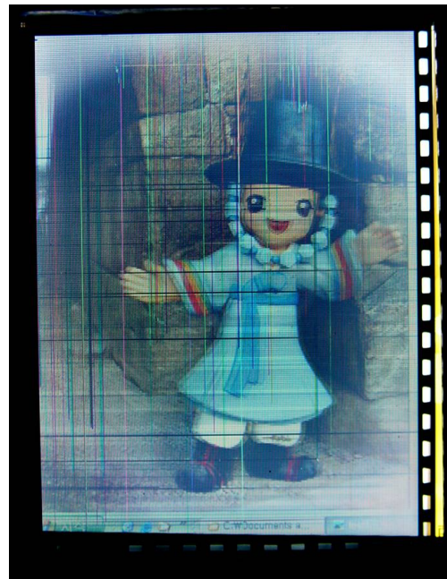
Figure 6. The photograph of an image displayed on a 5.5 inch stereoscopic display using WGP containing rows of alternating polarization angle.
