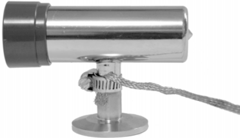
Figure 3-10 Grounding a Convectron Gauge
