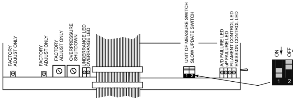
Figure 4-1 Ion Gauge Electrometer Module Top View
