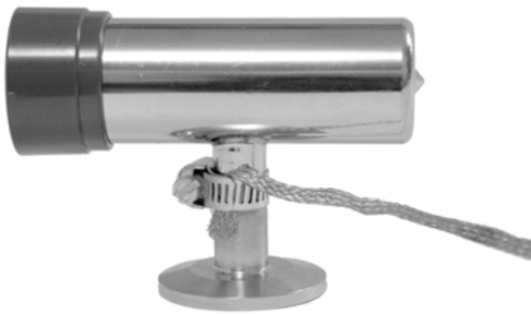
Figure 2-8 Grounding a Convectron Gauge
