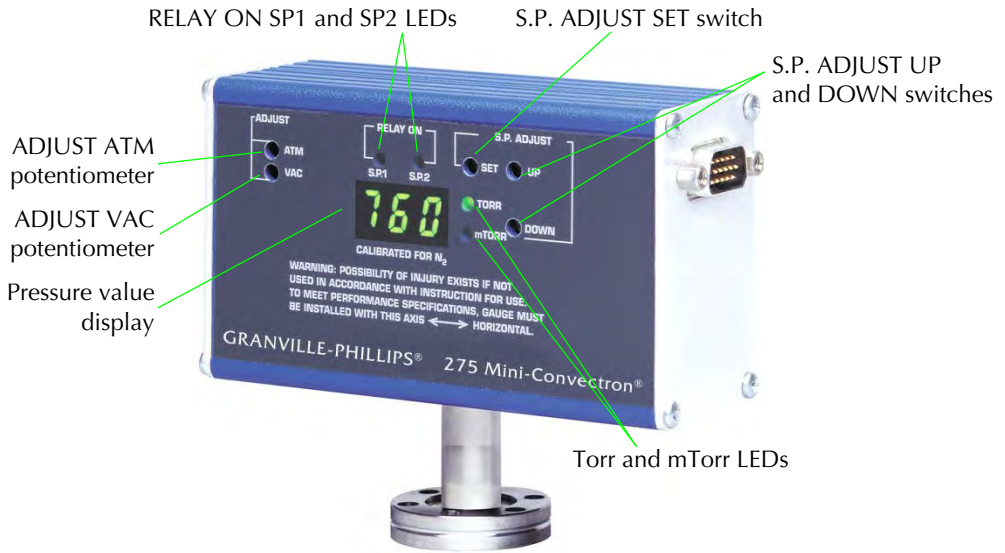
Figure 3-1 Mini-Convectron Module with two Setpoint Relays and 3-Digit Display
