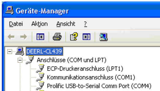
Device Manager showing the virtual driver for USB „Prolific“ at COM 4
