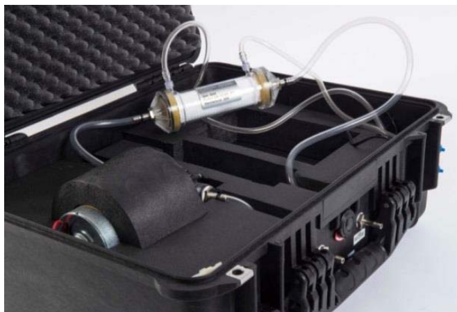
Figure 54: Interior view of REM1 with water pump, tubing and the REM module itself
