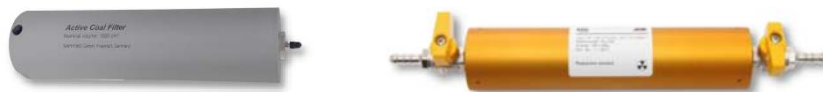
Figure 59: 1 L active coal filter for low level tests (left) and radon calibration source, traceable to the Czech Metrology institute (right)
