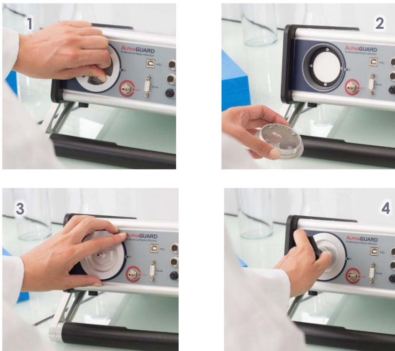
Figure 50: Exchanging the diffusion and the flow through adapters
