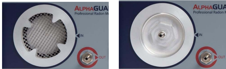
Figure 8: Air inlet with adapter for diffusion mode (left picture) and for flow mode (just for AlphaGUARD DF2000, right picture)
