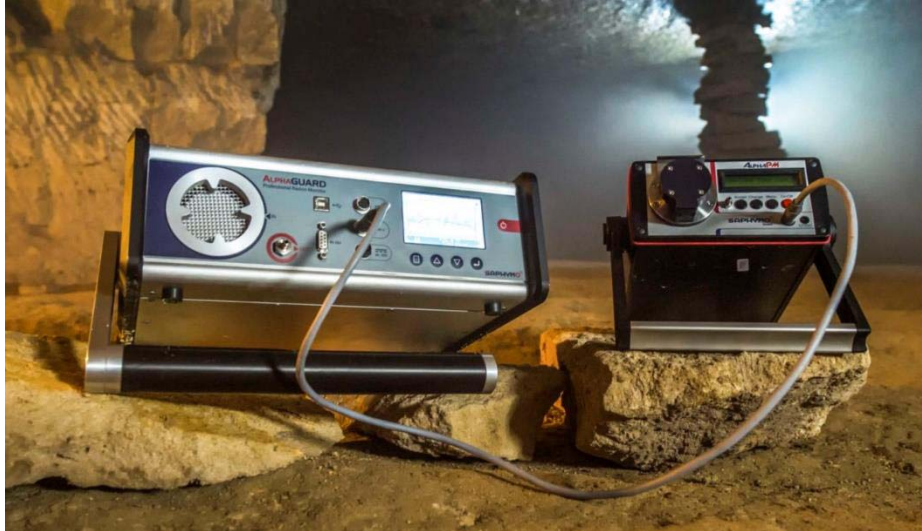
Figure 51: AlphaPM connected as front-end to AlphaGUARD for simultaneous monitoring of radon and its decay products
