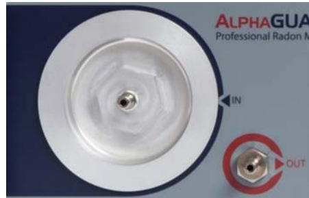
Figure 49: Air inlet with mounted flow through adapter for connecting tubes
