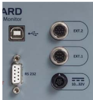
Figure 7: AlphaGUARD – electrical connections
