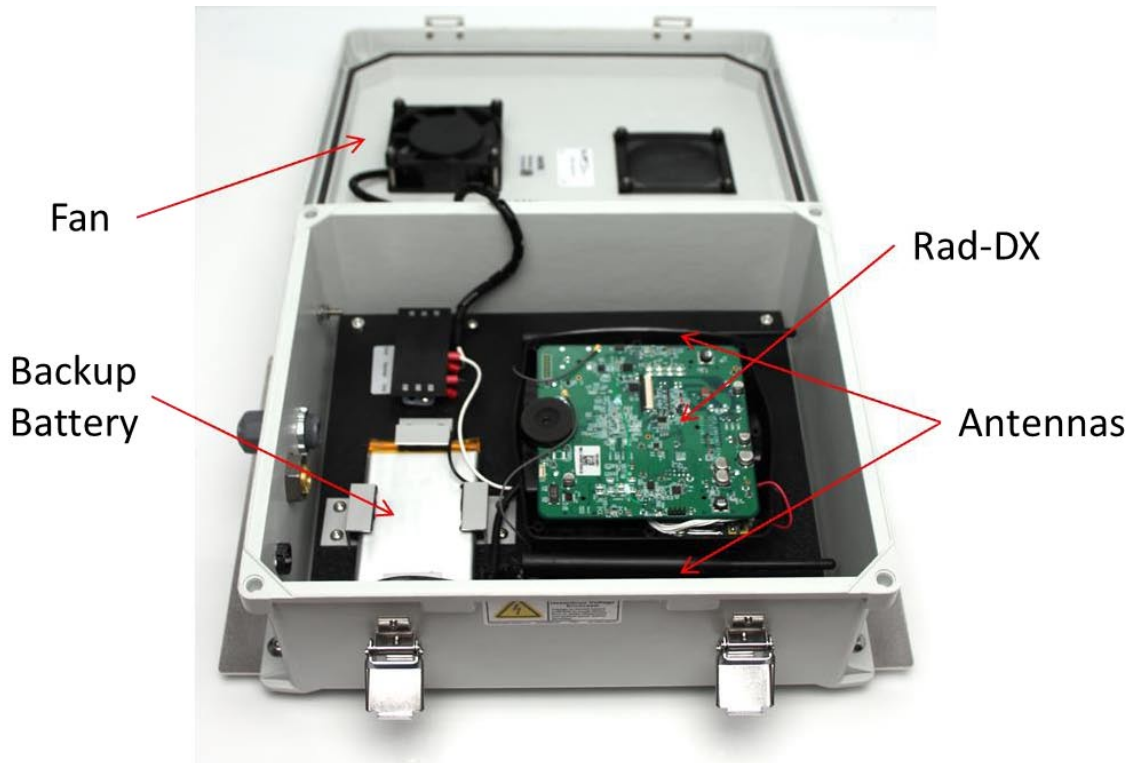
Figure 5: Inside the NEMA Enclosure
