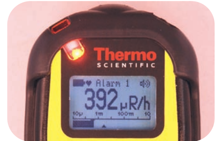
Alarm level 1 exceeded "Alarm 1" sign and "speaker" sign show up Absence of trend arrow indicates stable radiation level - reading can be taken
