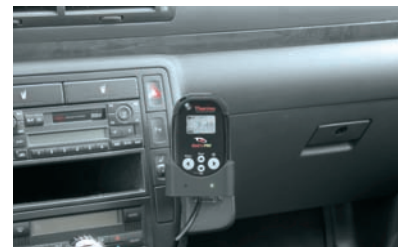
RadEye dash board adapter for mobile area survey applications including optional charging of the batteries
