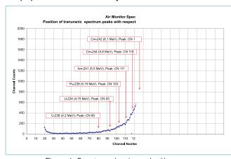
Figure 1: Spectrum showing radon/thoron interference and transuranic peaks.
