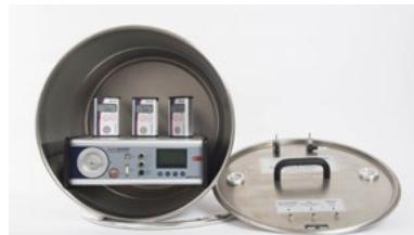
In combination with the radon chamber, AlphaGUARD allows the measurement of radon in material and the calibration of any other radon instruments
