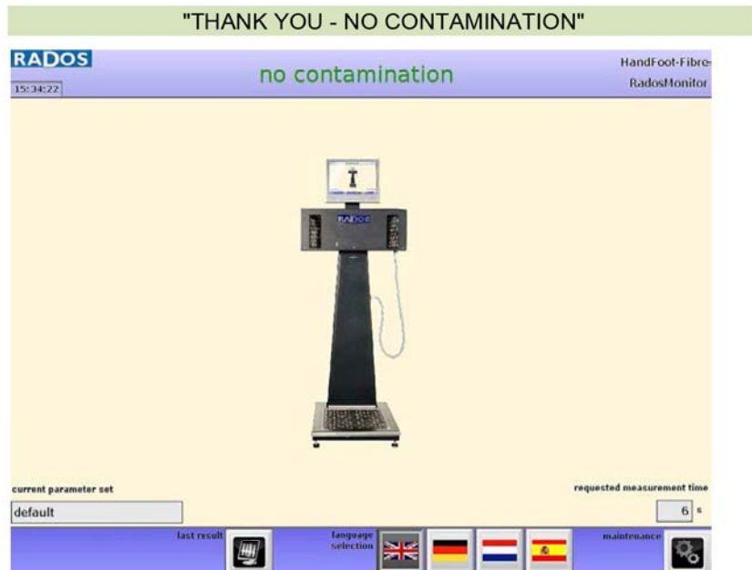
Figure 3-16: Display "no contamination"
