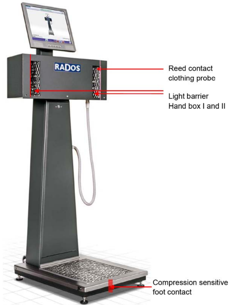
Figure 8-7: sensory location on the HandFoot-Fibre™
