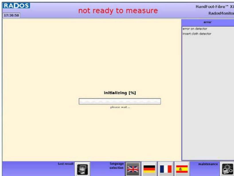
Figure 9-2: Failure - not ready to measure
