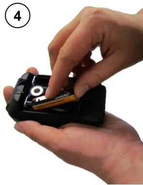
Insert two AA batteries into the AccuRad PRD. Ensure the correct polarity position.
