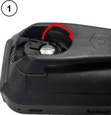
Release the battery cover tab.
