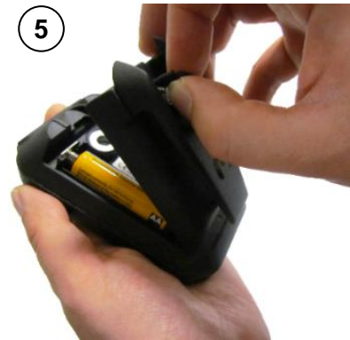
Reinstall the battery cover. Turn the cover tab clockwise to lock it.
