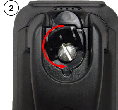
Turn counterclockwise the battery cover tab.
