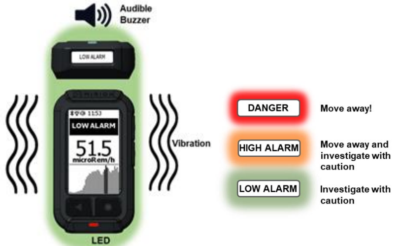
The AccuRad alarms when a source is detected. The operator presses any button to acknowledge the alarm and responds accordingly.
