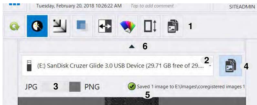
Figure 9-5: Scan Monitor mode or Review View mode screen (typical) after image export. (1) Export button to initiate export process (opens or closes the export subscreen), (2) Destination data store, (3) Target file format selection, (4) Export button to create files, (5) Acknowledgment notification with destination folder path, and (6) Close export subscreen button.
