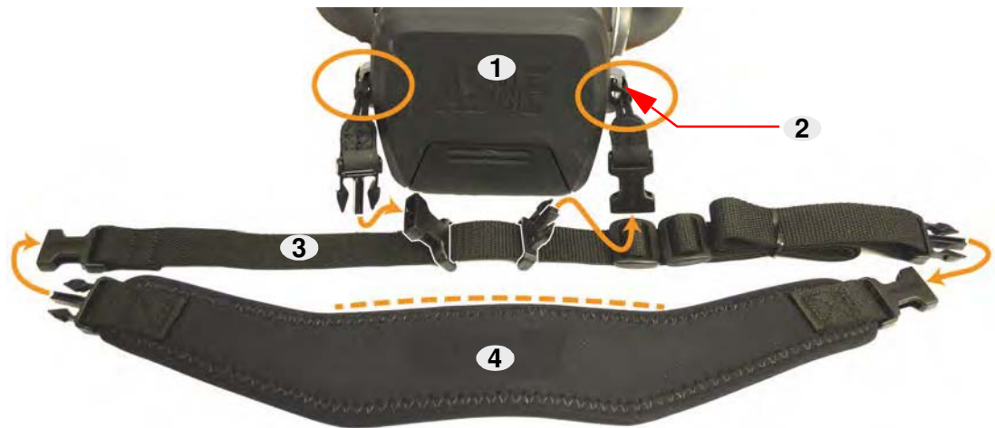
Figure 11-3: Shoulder Strap Assembly. The dashed line indicates the straight middle side of the Shoulder Pad, the side that is worn toward the operator's neck. (1) Rear of scanner unit, (2) eyes on scanner, (3) Shoulder strap with the two ends of the loop connectors already attached, and (4) Shoulder strap pad.
