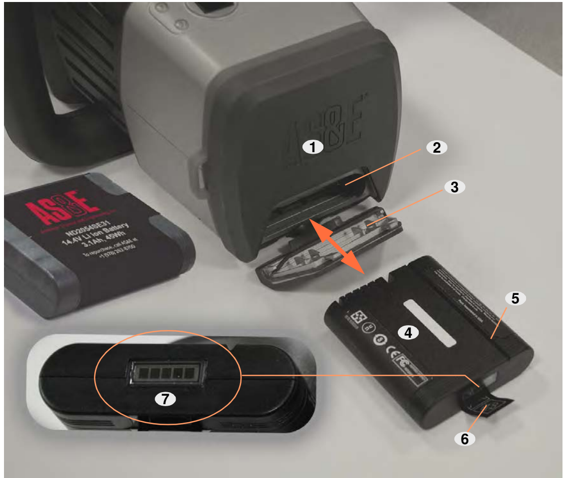
Figure 12-6: Scanner Battery Access. (1) scanner housing (rear view), (2) battery compartment (open), (3) tethered cover, (4) battery with (5) alignment groove, and (6) flexible tab (for removing battery from compartment). Inset (7) shows the LCD display for state-of-charge (five segments showing steady color indicates 100% charge).
