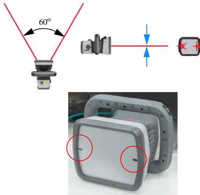
Figure 2-5: Dual laser beams visually indicate the X-ray beam path. The upper left panel shows the left-right beam fan angle of approximately 60°. The up-down fan angle is negligible, as indicated by the blue arrows in the upper middle panel.
