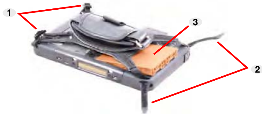
Figure 11-6: Hand Strap Position for Battery and Memory Card Access. (1) Buckle-type strips (for security), and (2) hook-and-loop strips (for easy loosening and tightening, during card and battery access). (3) Main Battery Pack, partially unloaded.
