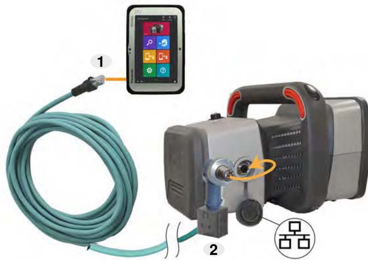
Figure 3-5: Ethernet Cabling Assembly (typical example). (1) Male Ethernet RJ-45 clip, (2) Ethernet right-angle (M12) plug with threaded ferrule.
