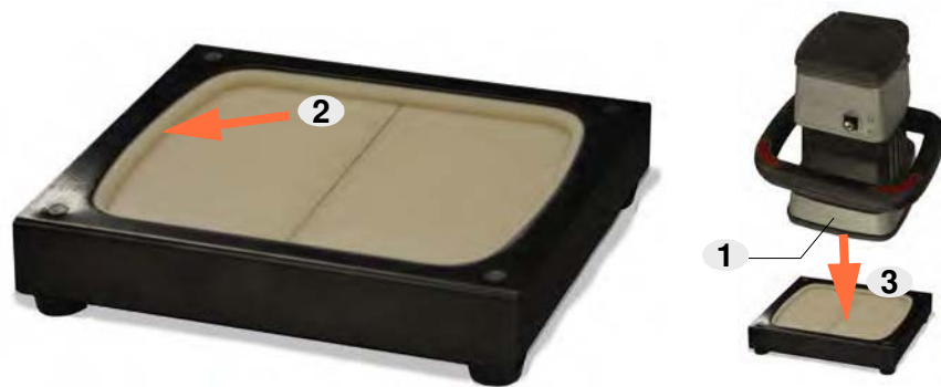
Figure 2-7: Calibration Dock application. (1) The MINI Z face is the section at the front of the scanner. (2) Alignment collar in the dock. Place the dock on a horizontal surface, with the four mounting feet downward. (3) Seat the Scanner Unit face down into the dock, making sure the front face of the scanner rests uniformly against the inside of the dock mounting collar.
