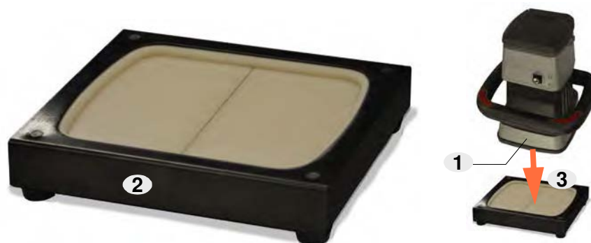
Figure 11-9: Calibration Dock application. (1) The MINI Z face is the section at the front of the scanner. (2) The dock itself is configured like a small block with a shallow alignment collar. Place the dock on a horizontal surface, with the four mounting feet downward. (3) Seat the face down into the dock, making sure the front face of the face rests uniformly against the inside of the dock mounting collar.
