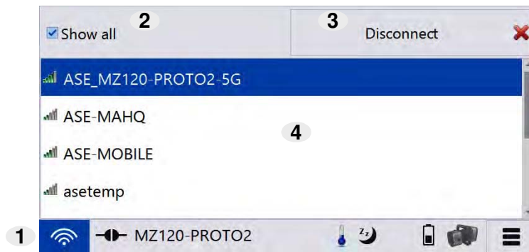
Figure 3-12: WiFi Connection list with a previously selected and connected scanner indicated. (1) WiFi Connection button (at bottom corner of all screens; highlighted background indicates that the list is open), (2) Show all check box (tap to show all WiFi nodes detected, including nodes that are not MINI Z systems and MINI Z scanners with confidential SSIDs), (3) Disconnect button (tap to remove a current connection before making a new connection); when the “X” icon in the corner is red, the highlighted selection is the scanner currently connected, and (4) list of detected WiFi connections.
