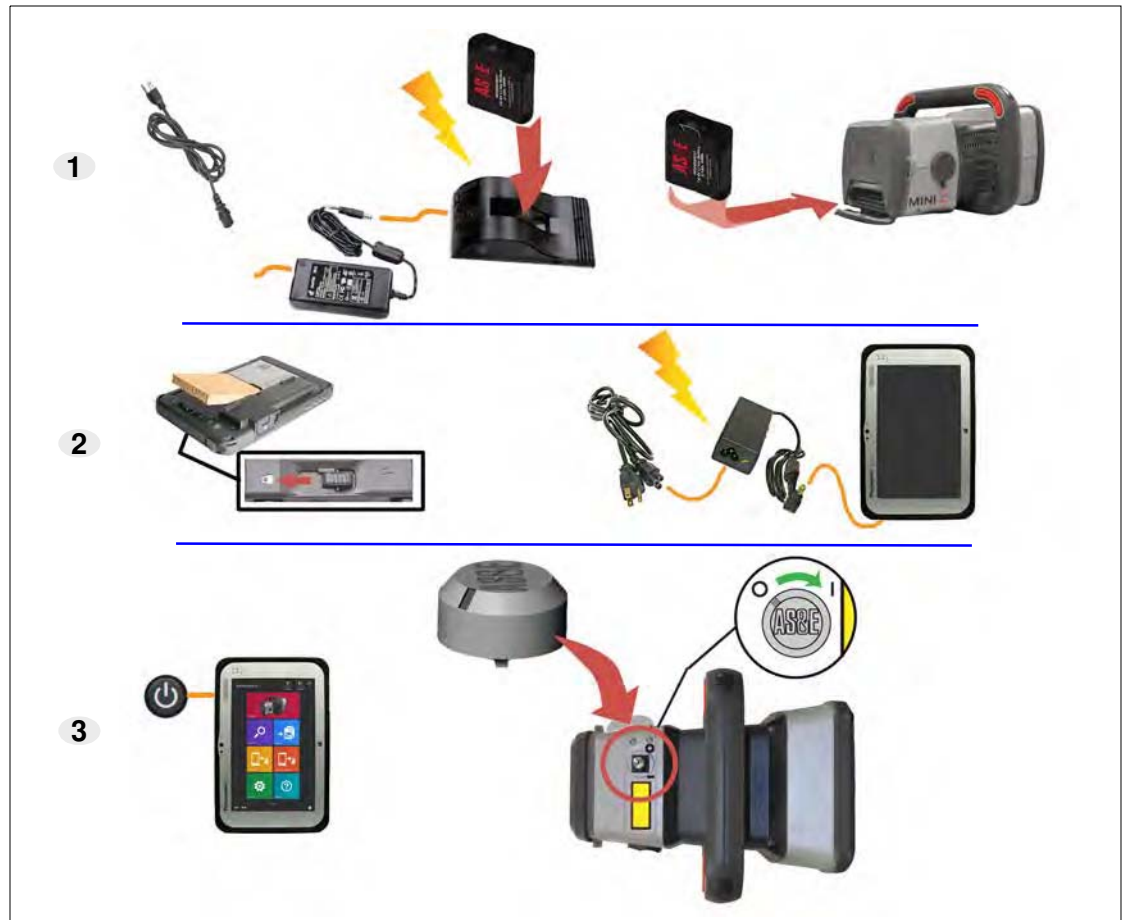
Figure 3-3: Quick Connection Guide (Not Using Ethernet Cable). (1) Assemble scanner battery charger and charge the scanner battery, then insert the charged battery into the scanner, (2) Insert battery into tablet, and assemble tablet battery charger and charge the tablet battery, (3) Push the Power button on the tablet; on the scanner, insert the key and turn toward ( I ) to power-on.
