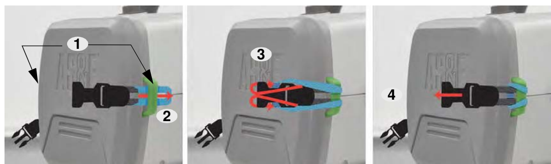
Figure 11-4: Shoulder Strap Loop Connector Male Side Assembly. (1) Mounting eye, one on each side of the scanner rear. (2) Male-side loop mounted through the eye, (3) over the clip, and (4) pulled tight.
