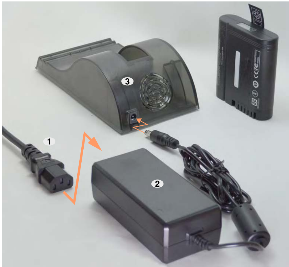
Figure 12-9: Scanner Battery Charger Setup. (1) one of three power cords (European, USA, and UK mains plugs), (2) AC adapter (3) charger.
