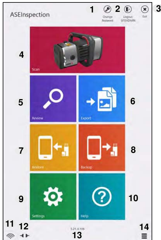
Figure 5-1: Home Screen Layout. Top-level screen of the MINI Z software. Tap individual buttons in the Content pane to open screens for controlling system functions. The buttons are described in Table 5-1 .
