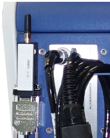
Fig. 20: Fasten the transmitter with Velcro in a free place
