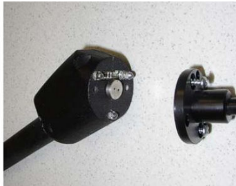
Fig. 19: Sinter filter in the sniffer handle
