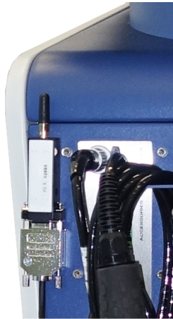
Fig. 21: The transmitter can be attached to a free spot with the supplied Velcro tape.
