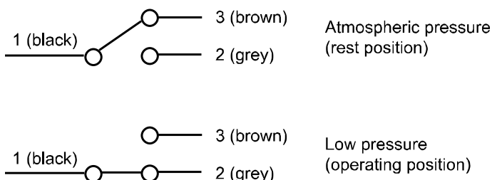
Fig. 2 Contact assignment of microswitch
