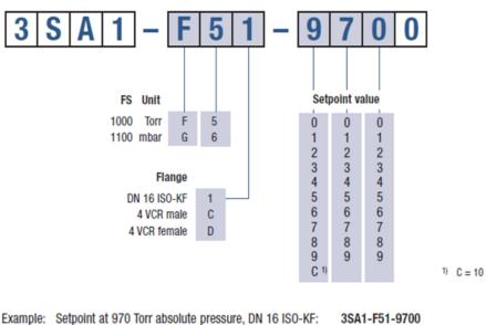
Example: Setpoint at 970 Torr absolute pressure, DN 16 ISO-KF: Setpoint at 1080 mbar absolute pressure, 4 VCR male:
