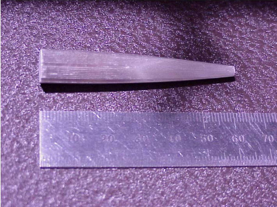
FIG. 47. Fibre-optical lens for neutron focusing [115, 116].
