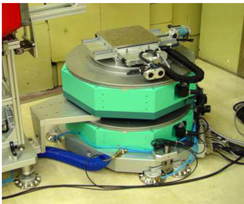
FIG. 11. Specimen positioning and rotation assembly as installed at the HFR in Petten, the Netherlands.
