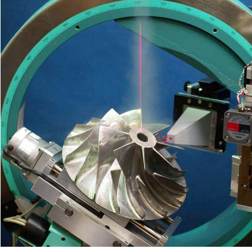
FIG. 12. Eulerian cradle carrying an impeller wheel at the E3 diffractometer at HZB Berlin.
