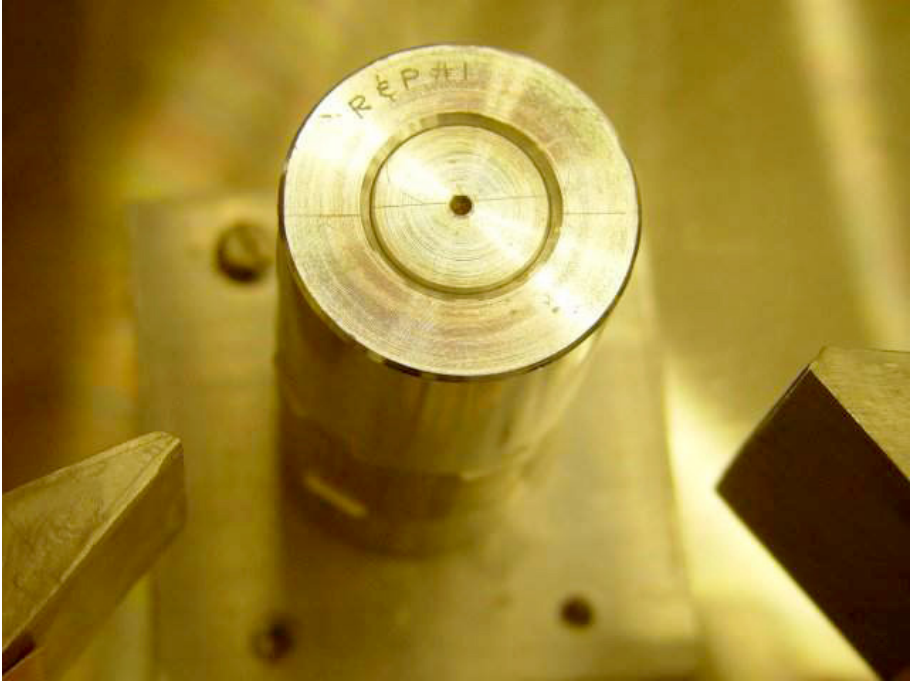
FIG. I-7. Round robin No. 2: Aluminium ring and plug specimen at neutron diffractometer, measurements in hoop direction (normal to the engraved fiducial mark).
