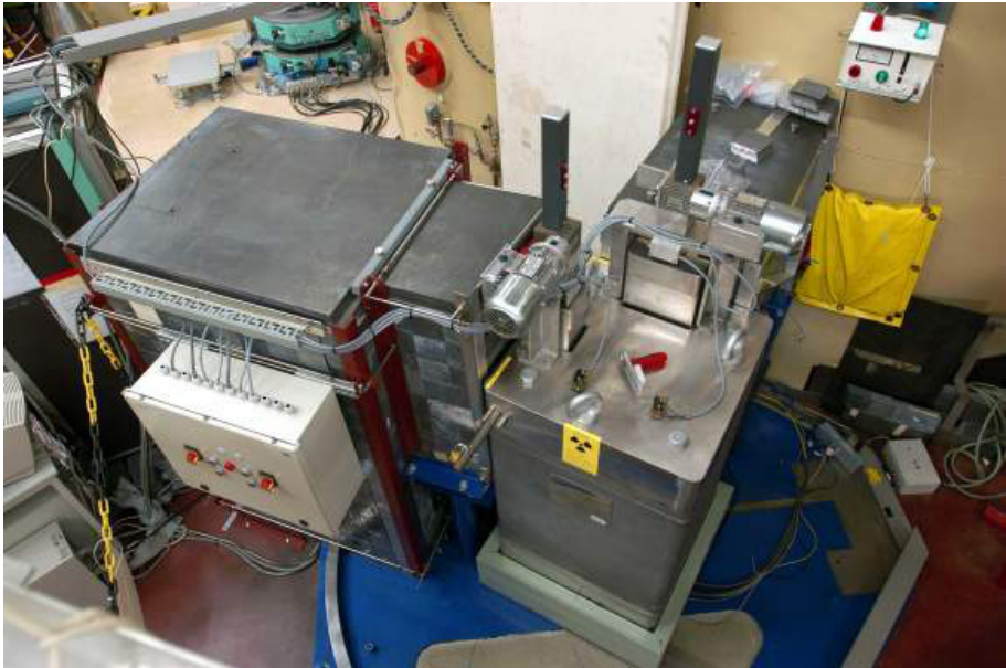
FIG. 18. Shielding installation for strain measurements in highly activated specimens.
