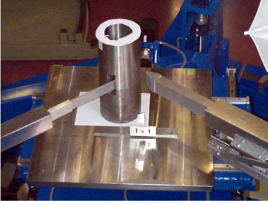
FIG. 35. Bimetallic piping weld specimen during hoop direction measurements at the HB4 Large Component Neutron Diffraction Facility at the HFR Petten. The incident neutron beam duct is on the left and the diffraction neutron beam duct is on the right. At the front end of the diffracted beam duct, the cadmium mask providing for the beam aperture can be seen.
