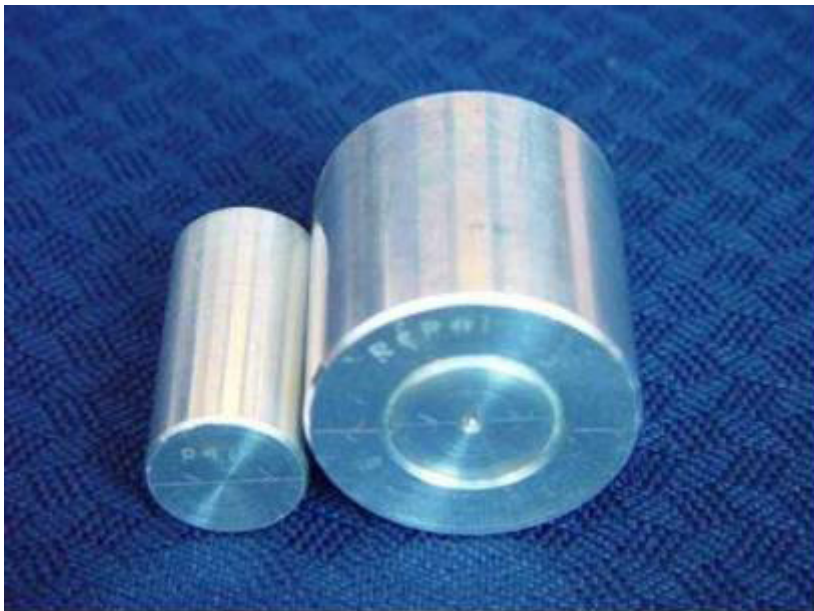
FIG. I-2. Round robin No. 1: aluminium ring and plug interference fit specimen set.
