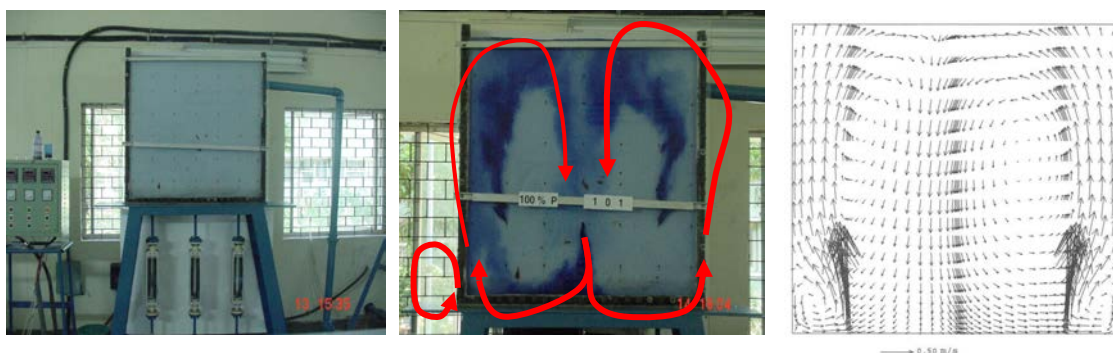
FIG. 6.30. Comparison of mixing characteristics of multiple jets in main vessel cooling system.
