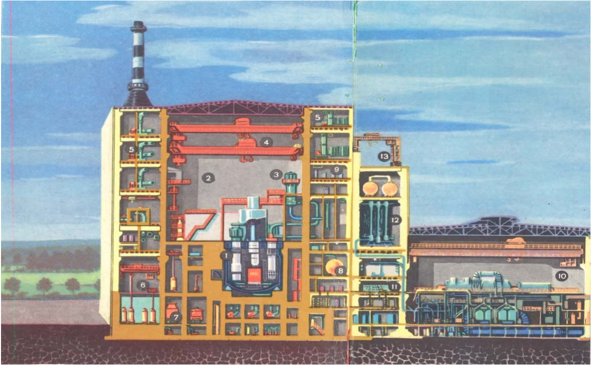
1-reactor, 2-reactor hall, 3-secondary pump, 4-crane, 5-ventilation system, 6-water pool, 7-irradiated fuel transfer cask, 8-sodium storage tank, 9-electric heating control system, 10-turbine hall, 11-control and protective system, 12-steam generator (SG), 13-crane (for SG)
