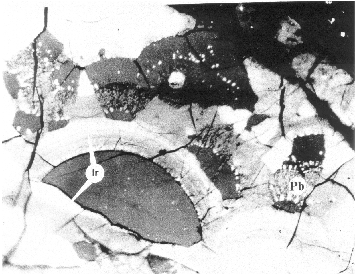
FIG. 9. U-Mo mineralization in hydromica metasomatites Argunskoe deposit (Spherulitic crusts of iordizite (Ir) with pitchblende (Pb) inclusions. Reflected light. Magnification 500).
