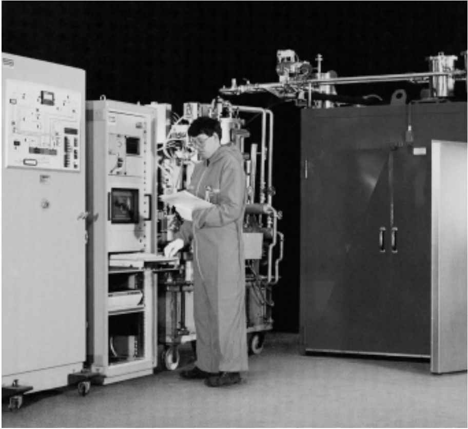
FIG. 30. PETRA facility for drying waste drums (Germany).
