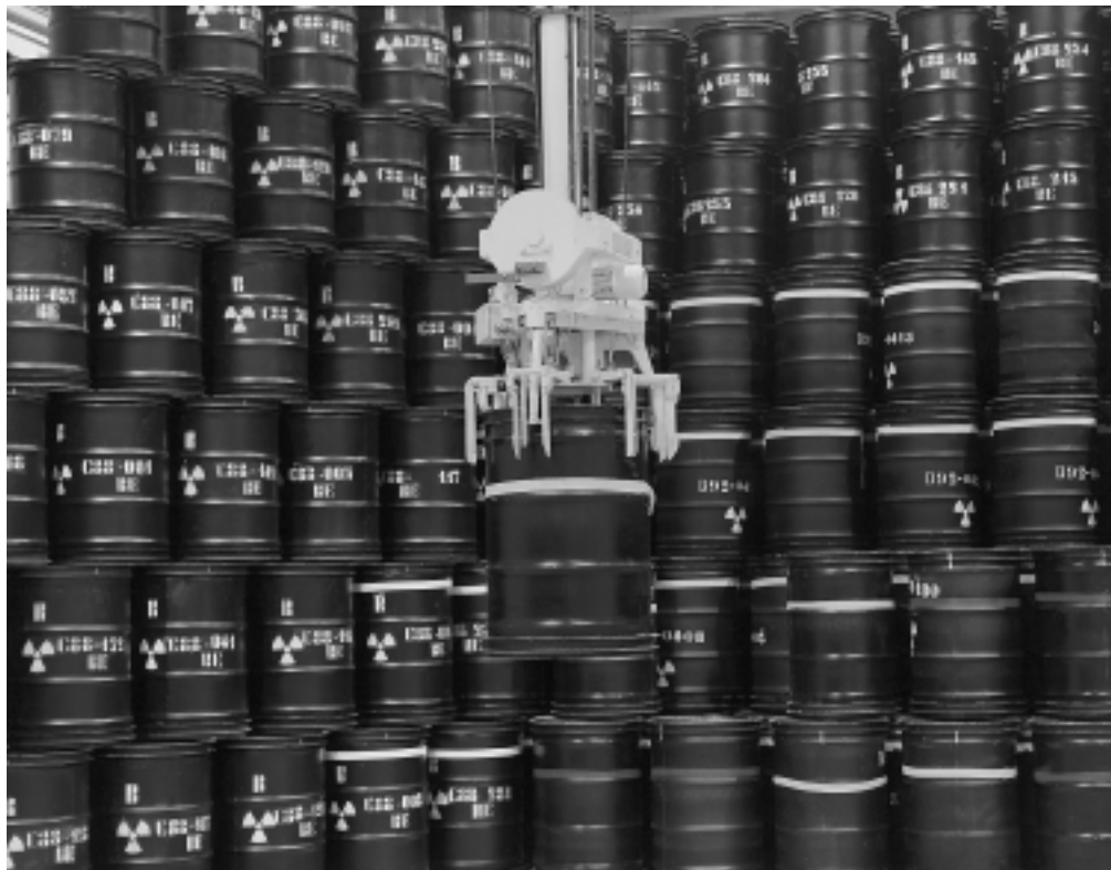
FIG. 15. Emplacement of drums in racks for stacking (Belgium).
