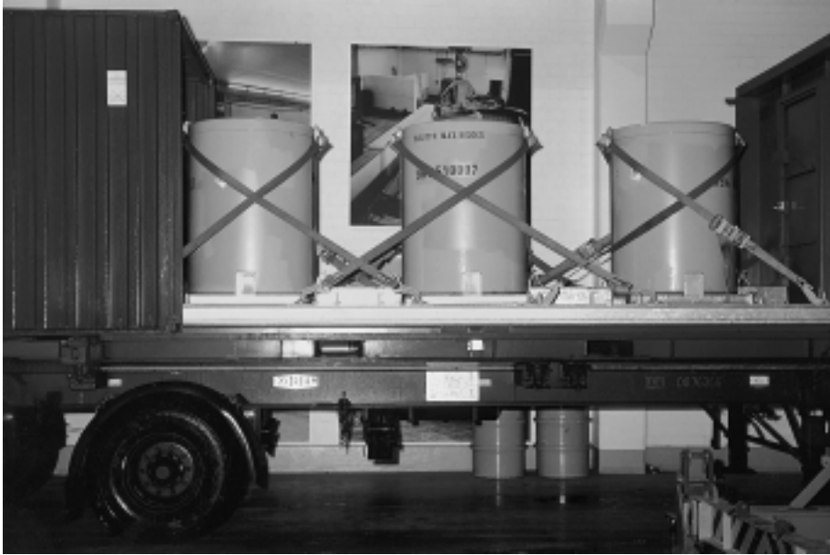
FIG. 6. Shielded cast iron cask, typically used for transport and storage of high dose rate LILW (Germany).
