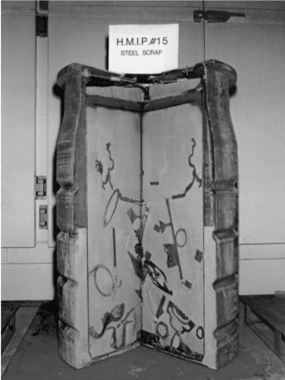
FIG. 2. Metallic scrap material embedded in cement (UK).
