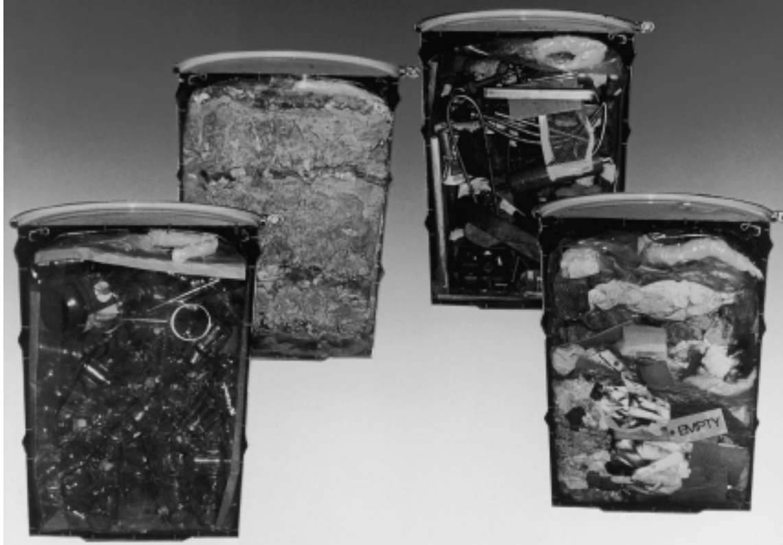
FIG. 1. Non-immobilized solid waste (glassware, evaporator solids, miscellaneous contaminated non-organic and organic equipment) in containers (USA).
