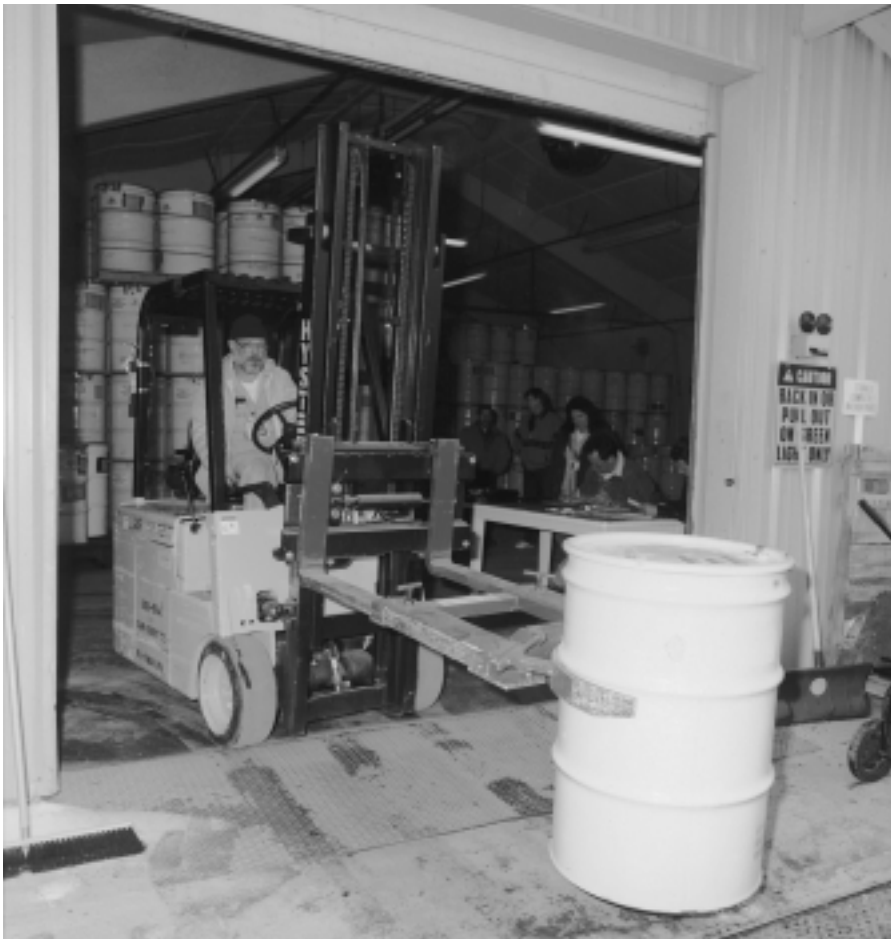
FIG. 12. Handling a 200 L drum with a lift truck (USA).
