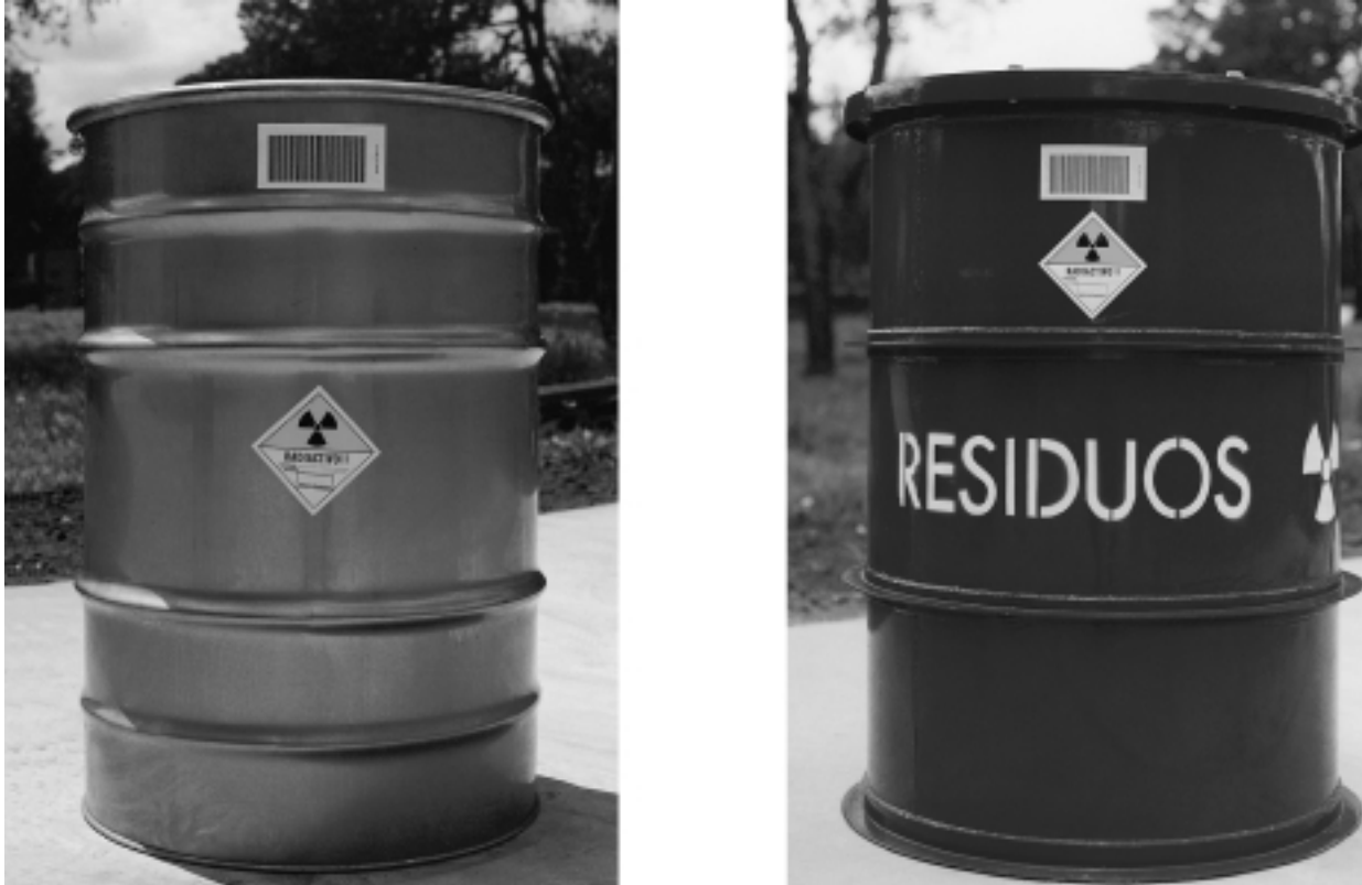
FIG. 3. Standard cylindrical drums used for packaging LILW (Argentina). Left: 200 L stainless steel drum; right: 400 L carbon steel drum with an epoxy paint inside and outside.
