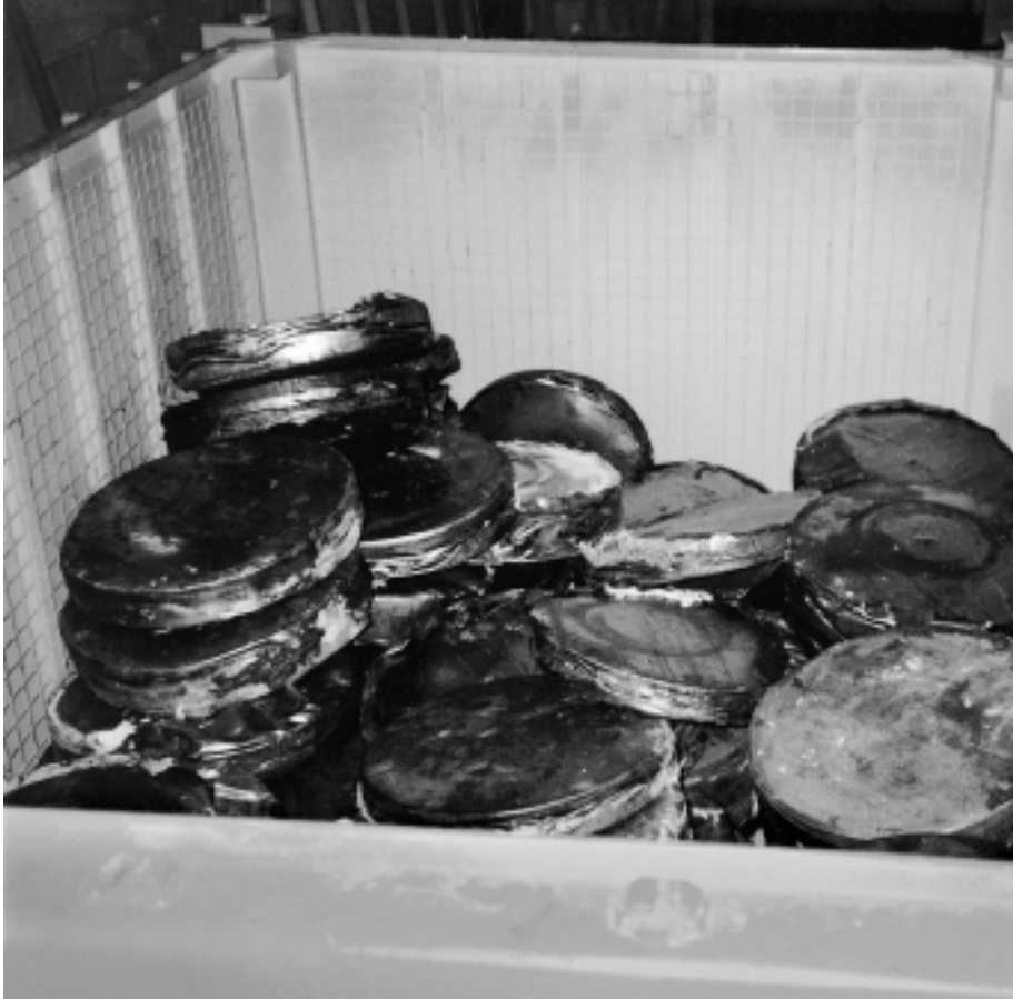
FIG. 8. View inside a steel container partly filled with supercompacted LILW pellets to be stored with or without grouting (Germany).
