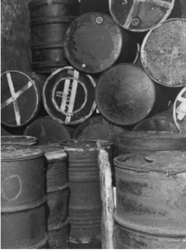
FIG. 28. Examples of corrosive failures of waste packages.
