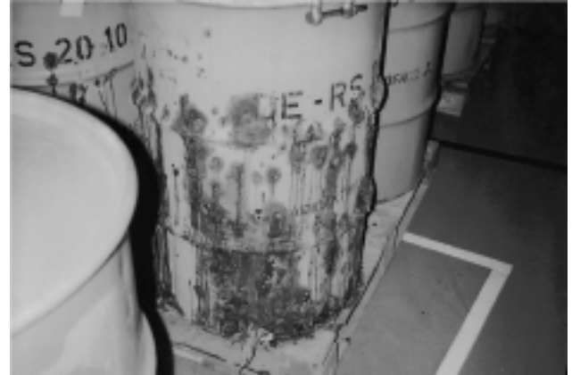
FIG. 28. Examples of corrosive failures of waste packages.
