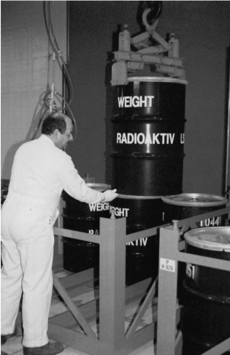
FIG. 14. Emplacement of a 200 L drum in the rack (Belgium).
