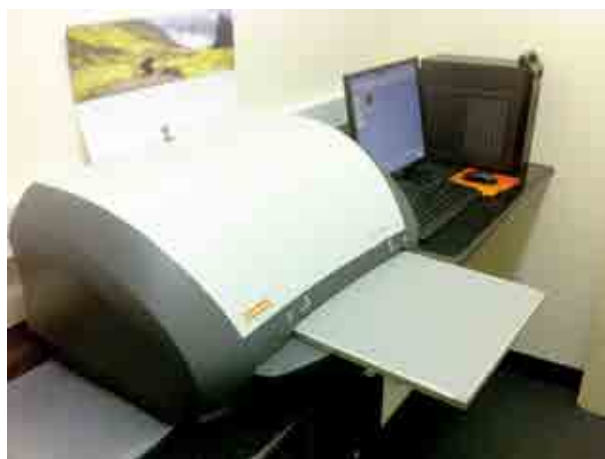
FIG. 11. Modern compact CR reader with quality assurance review station (also acts as patient ID station) and imaging plate (photograph courtesy of W. van der Putten, Ireland).
