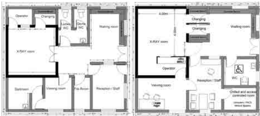
FIG. 7. An example of remodelling of a small X ray suite to go from film based to digital X ray. On the left is the facility before conversion to digital imaging. The introduction of digital technology has also improved workflow functionality through a limited removal of existing walls.
