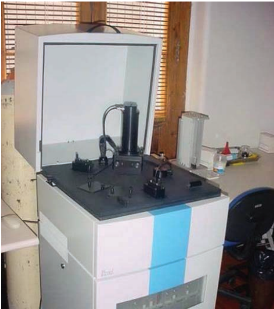
FIG. I-2. (a) Fimel PCL3 TL reader and (b) Landauer InLight MicroStar OSL reader.
