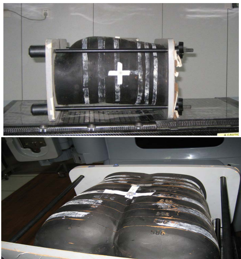
FIG. IV-6. Alderson phantom set-up for pelvic measurements.
