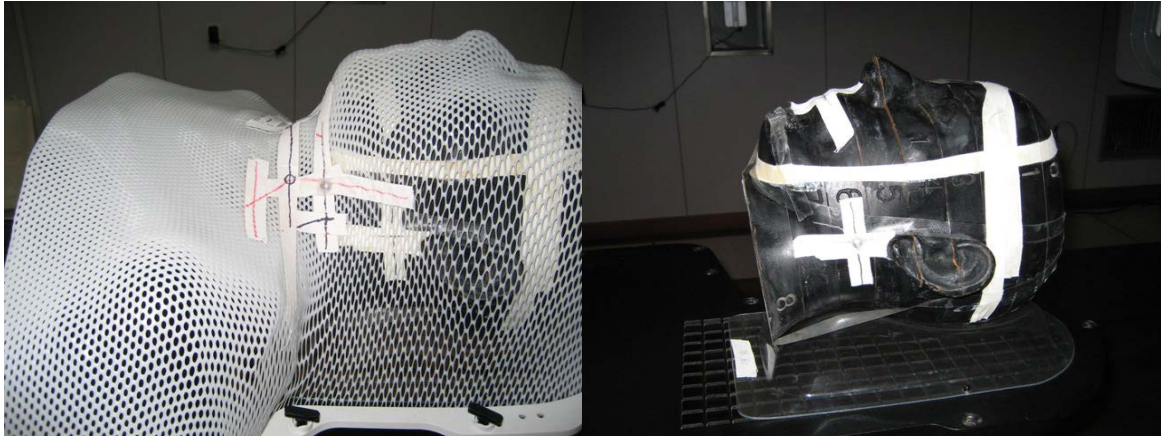
FIG. IV-8. Alderson Rando phantom set-up for head and neck measurements.
