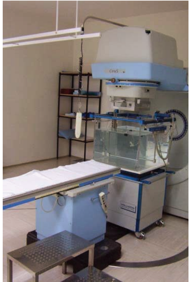
FIG. III-1. (a) Diode holder on the rails; (b) ^{60}\text{Co} unit with a water phantom.
