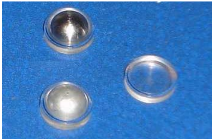
FIG. 7. TLD buildup caps of aluminium (left bottom) used for measurements in a ^{60}\text{Co} beam and of stainless steel (left top) used for TLD measurements in 6 MV and 15 MV high energy photon beams. A 1 mm thick PMMA baseplate used for TLD encapsulation is also shown (right).
