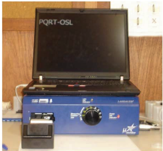
FIG. I-2. (a) Fimel PCL3 TL reader and (b) Landauer InLight MicroStar OSL reader.
