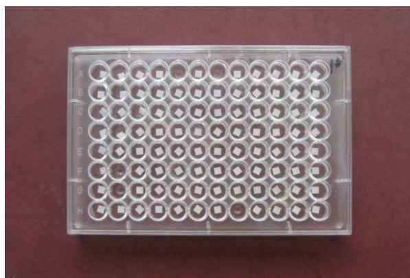
FIG. IV-4. Plastic box used to house TLDs.
