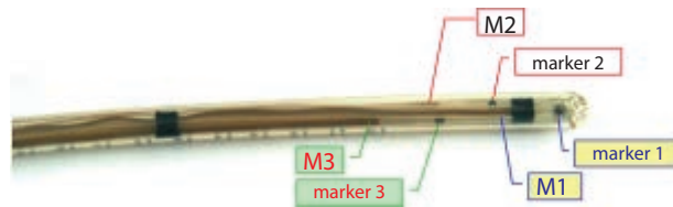
FIG. V-3. Rectal probe composed of three MOSFET dosimeters.
