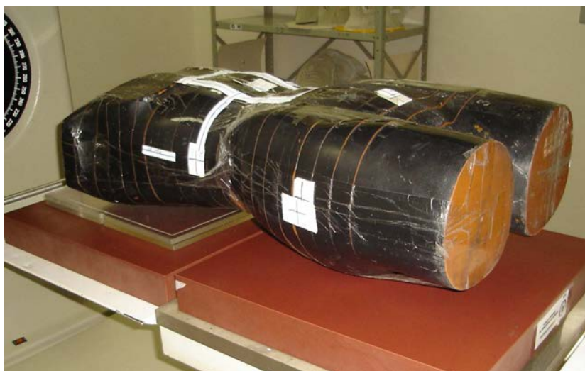
FIG. I-3. The female Alderson Rando anthropomorphic phantom used in the project.
