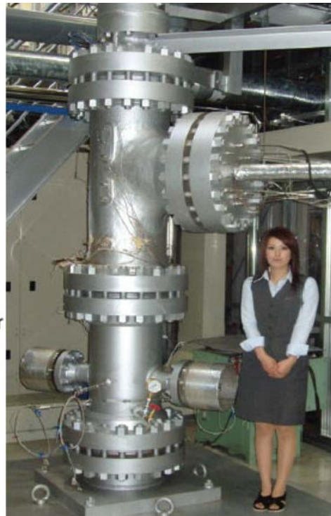
FIG. 169. Schematic of JAEA high temperature isolation valve concept (left), half scale model (right) [385].
