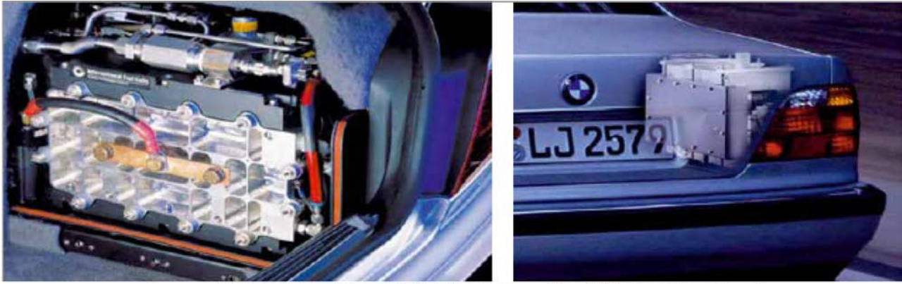
Power: 5 kW(e), Voltage: 42 V, Efficiency: 35 - 40% (total system) Volume: 20 l (stack) and 48 l (total), Weight: 22 kg (stack) and 45 kg (total)
