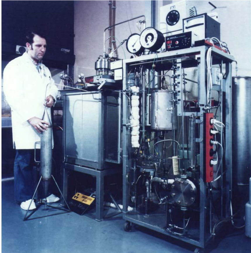
FIG. 147. Test facility AUWARM of FZJ for measurements of hydrogen permeation.
