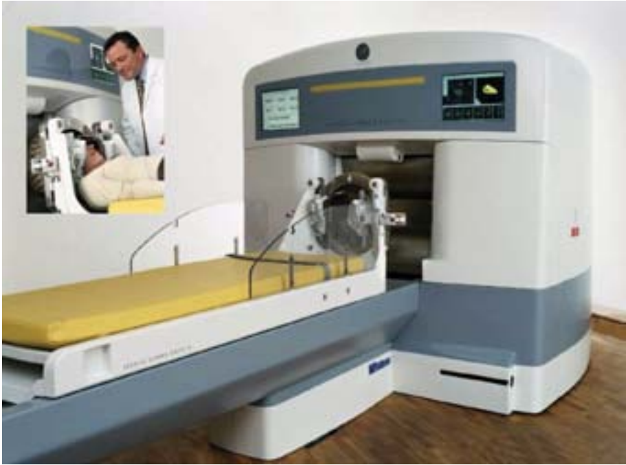
FIG. 15.1. State of the art Gamma Knife (Model 4C) showing the main body of the unit containing 201\ ^{60}\text{Co} sources (each nominally with an activity of 30\ \text{Ci} = 1.11 \times 10^{12}\ \text{Bq} ), the treatment table and a collimator helmet deployed for treatment. The inset shows an up-close image of the automatic positioning system used to position the patient for treatment. (Courtesy of Elekta AB.)
