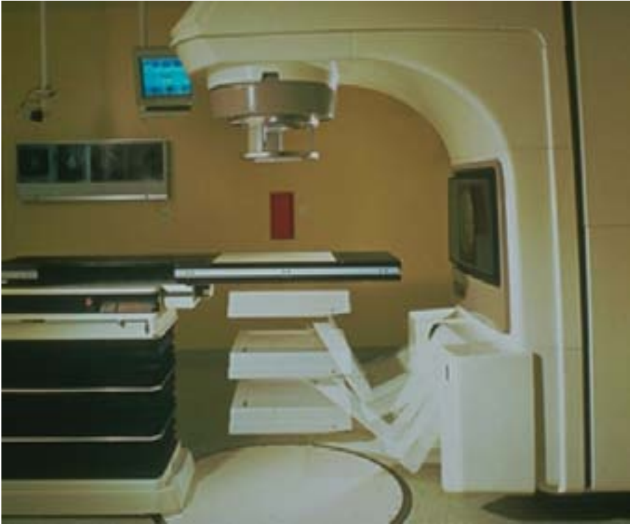
FIG. 12.2. Liquid filled matrix ionization chamber type of EPID connected via a retractable arm to a linac.
