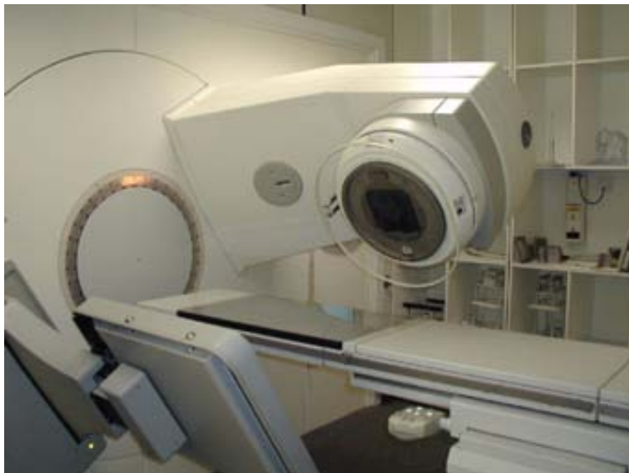
FIG. 12.3. Amorphous silicon type of EPID installed on the gantry of a linac.
