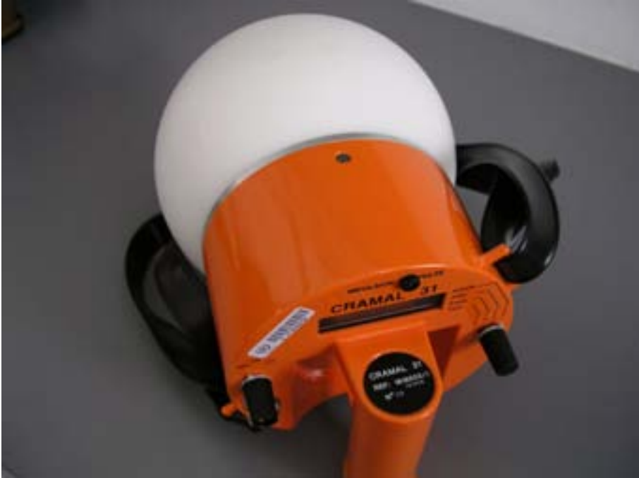
FIG. 4.3. Neutron dose equivalent rate meter with a thermalizing polyethylene sphere with a diameter of 20 cm.
