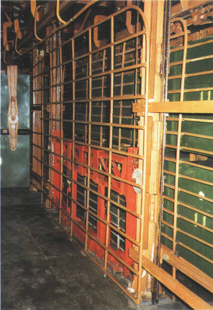
Photograph 1. Source rack frame and protection grid. The orange metal frame is the upper part of the shielding plug for the source rack. Spaces at both sides of the frame allow the counterweights to slide down.
