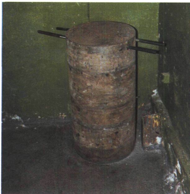
Photograph 7. Lead shielded gamma monitoring probe inside the irradiation chamber.
