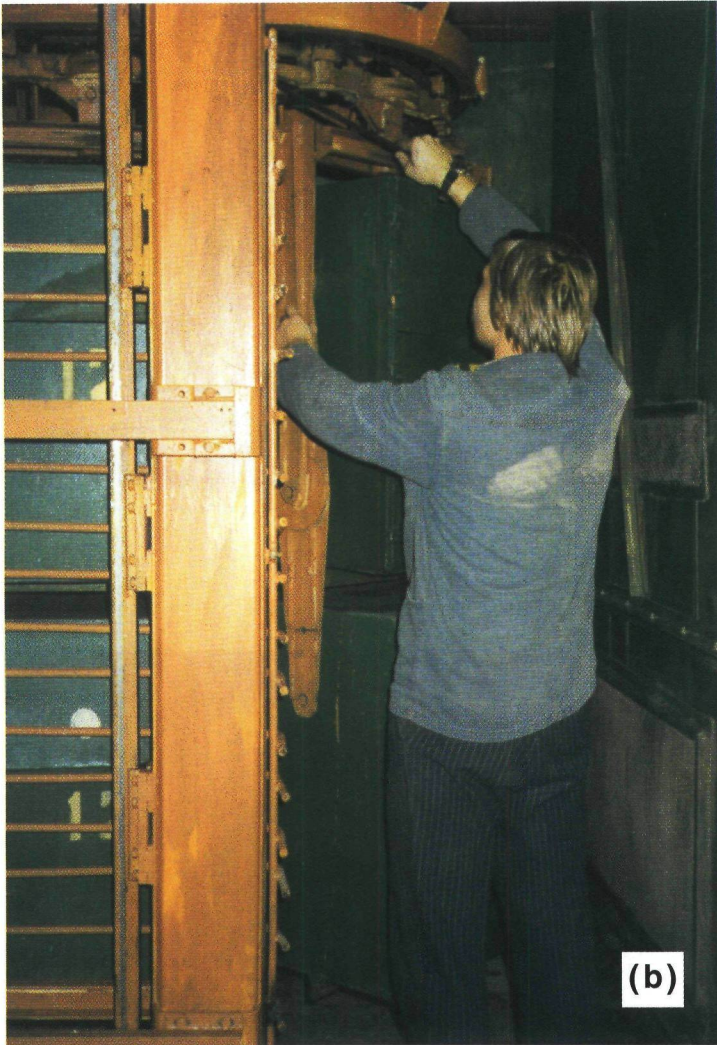
(b) trying to release the jammed carriage couplings.
