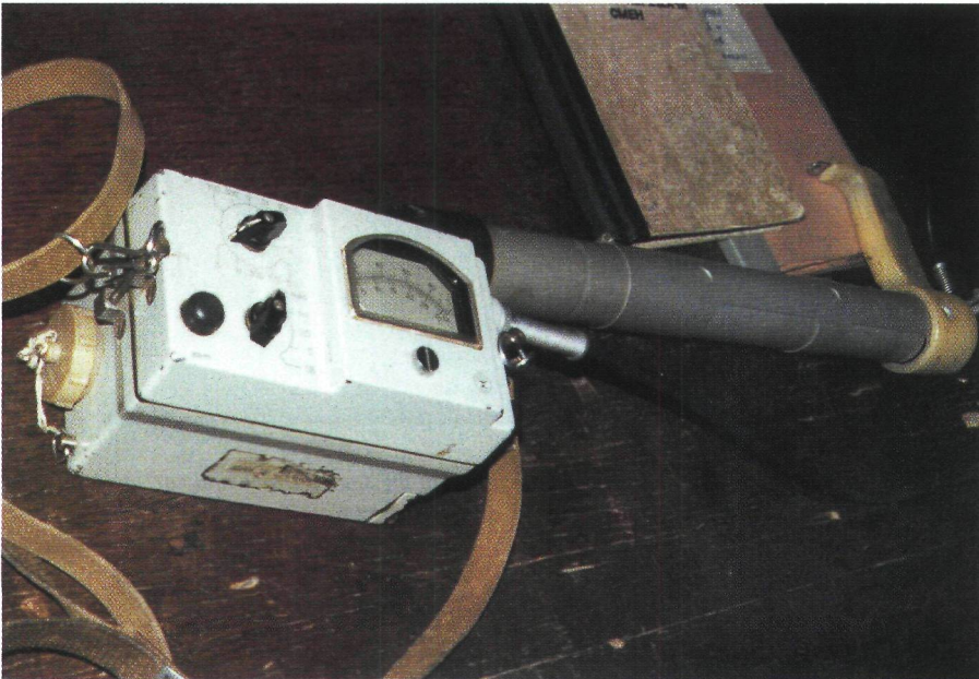
Photograph 10. Portable dose rate monitor used during the entry procedure.
