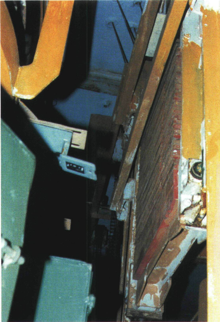
Photograph 2. Counterweight in the upper position (source in the shielded/storage position).
