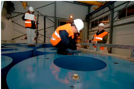
FIG. 9. Examples of seals that are used by the IAEA to maintain continuity of knowledge.
