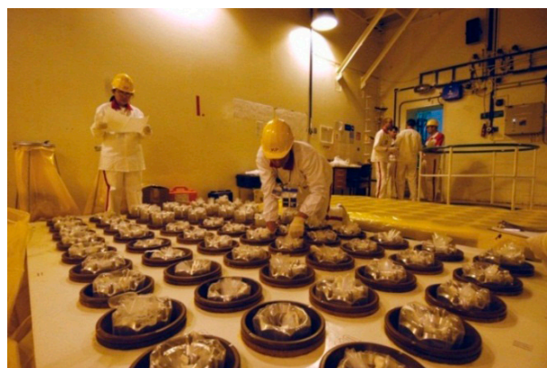
FIG. 4. Item counting in a fresh fuel store.
