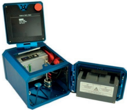
FIG. 7. A next generation IAEA surveillance system.
