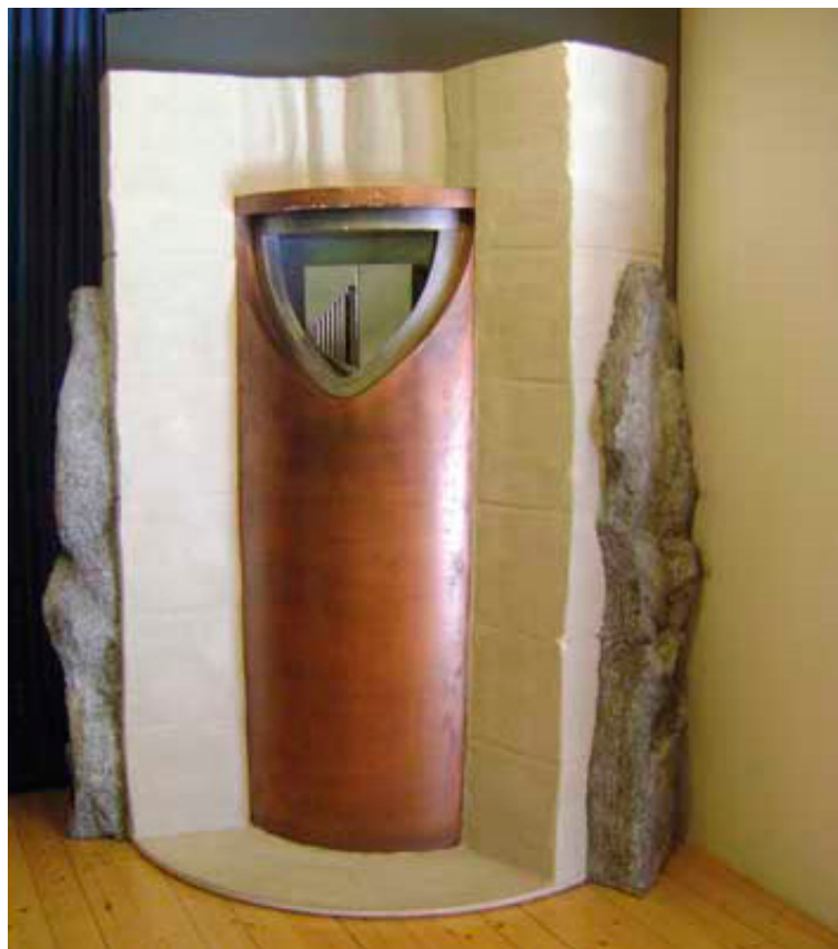
FIG. 22. Cut-away model of a canister for encapsulating spent fuel in a geological repository.
