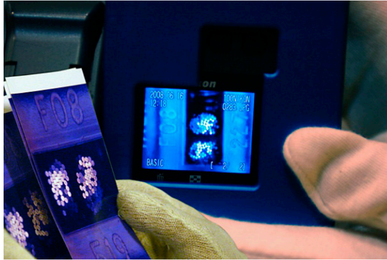
FIG. 12. Example of a fibre optic seal being interrogated.
