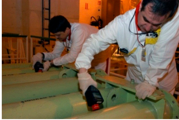
FIG. 5. Verification of fresh fuel transport containers using a handheld HM-5 gamma monitor.
