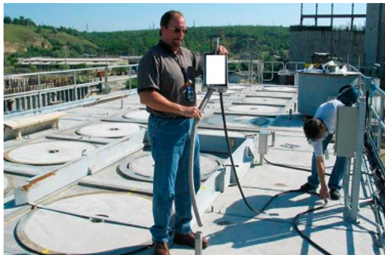
FIG. 21. IAEA inspector installing unattended monitoring on MACSTOR-200 facility.
