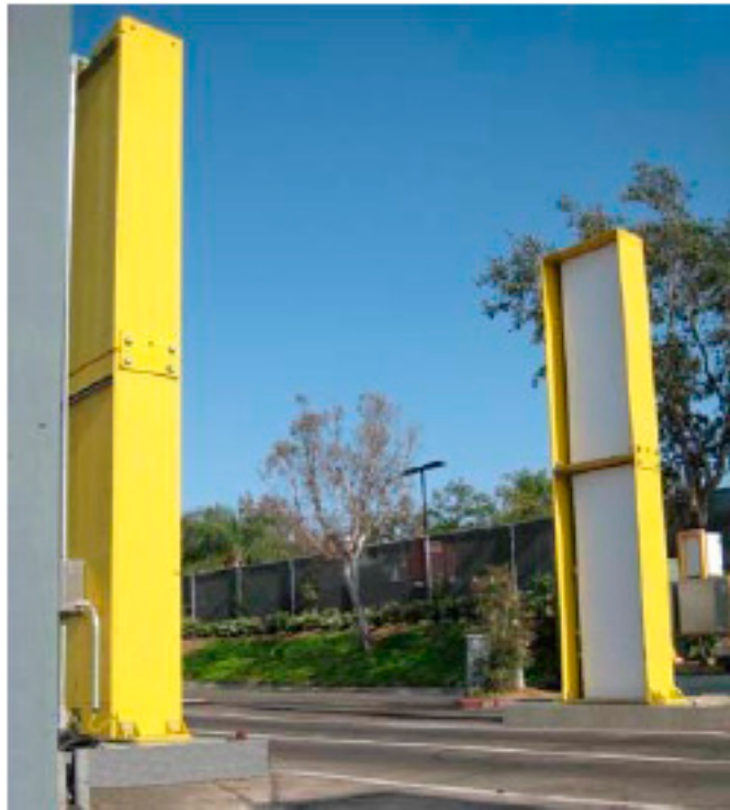
FIG. 23. Radiation portal monitors placed at a repository entrance.
