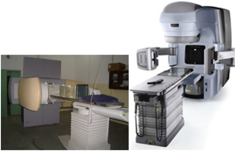
FIG. 8.9. A modern cobalt teletherapy unit and a radiotherapy linear accelerator. Portal imaging using film on the cobalt unit shown here and, similarly, an electronic device on the accelerator, are used to verify patient and target volume position relative to the equipment isocentre, prior to treatment. The accelerator is also fitted with an orthogonal X ray imaging system (images courtesy of the IAEA Programme of Action for Cancer Therapy and Varian).
