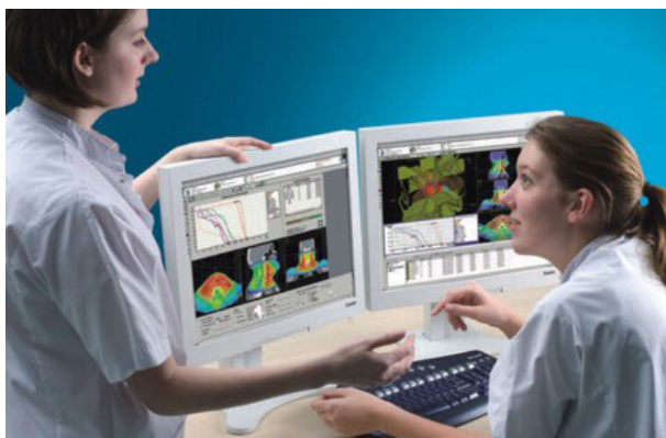
FIG. 8.7. A TPS workstation showing reconstructed images of the patient's anatomy, radiotherapy beam portals, isodoses and plan evaluation tools (images courtesy of Elekta).
