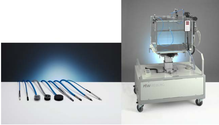
FIG. 8.14. Waterproof detectors (left) are used to measure relative dose profiles in computer controlled beam acquisition systems, which are large water phantoms (right) (images courtesy of PTW).
