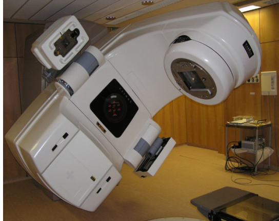
FIG. 9.4. A linac commonly used in radiosurgery (image courtesy of Varian Medical Systems).
