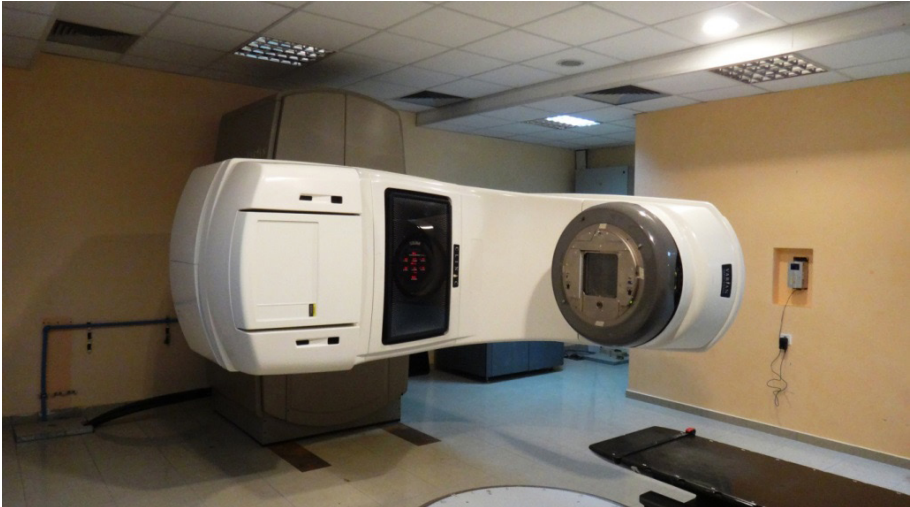
FIG. 28.2. Modern medical linac for cancer treatment. (Photo courtesy of the National Oncology Centre, Nouakchott, Mauritania.)
