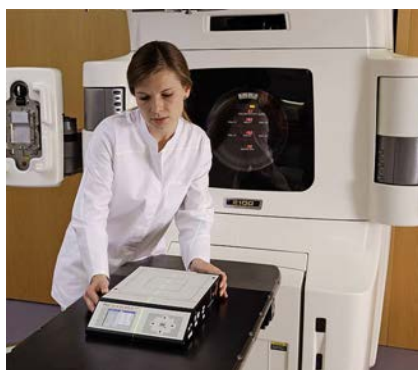
FIG. 8.12. A medical physicist positioning a check device on the treatment couch of a linear accelerator in order to carry out a quality control check of the beam (image courtesy of PTW).
