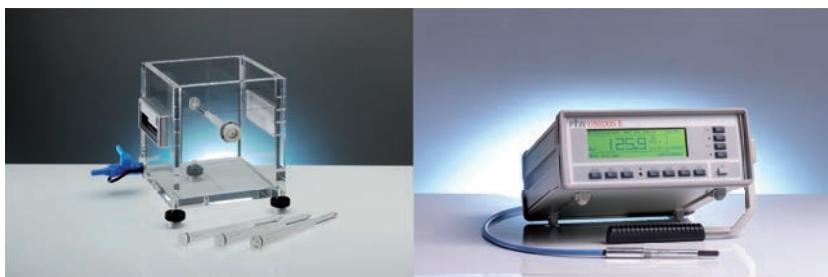
FIG. 8.13. A water phantom and an absolute dosimetry system (ionization chamber and electrometer) that is used to determine the reference output of megavoltage photon beams from a teletherapy treatment unit. Such systems are calibrated by a dosimetry standards laboratory that has been accredited to provide an internationally traceable coefficient (image courtesy of PTW).
