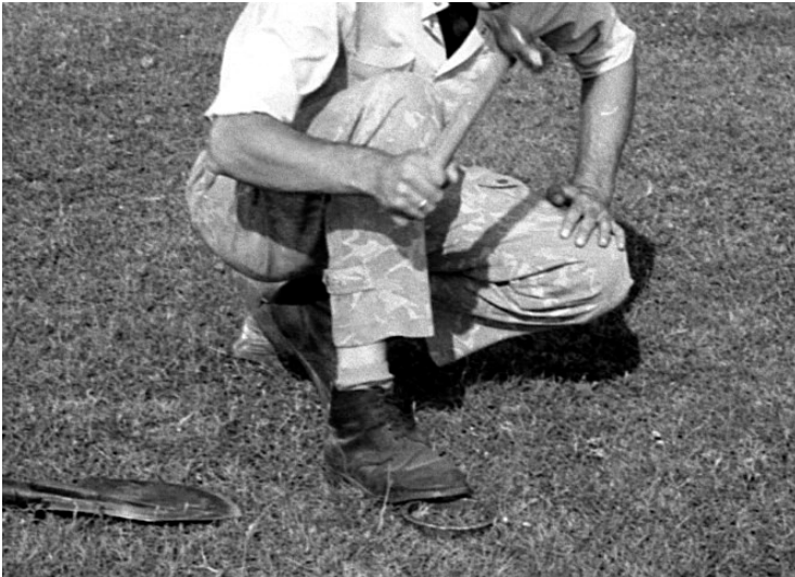
FIG. 8.2. Sampling with a 14 cm ring. (Courtesy of Ukrainian Institute of Agricultural Radiology.)
