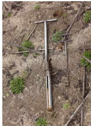
FIG. 8.7. Sampler with a diameter of 37 mm (0.001 m 2 ).
