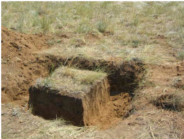
FIG. 8.41. Study using the monolith method. (Courtesy of V. Kiznetsov, Russian Institute of Radiology and Agroecology, Obninsk.)
