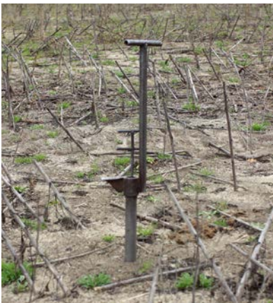
FIG. 8.7. Sampler with a diameter of 37 mm (0.001 m 2 ).
