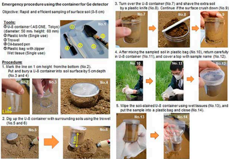
FIG. 8.19. Emergency procedure for the investigation of radioactive contamination of the soil using the U-8 container.
