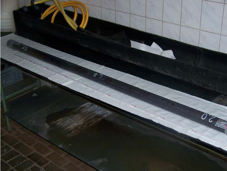
FIG. 4.5. Undisturbed liner sample (100 mm in diameter and 2 m long) of soft tailings obtained below water table using hand operated corer sampling equipment (0.2 m deep).
