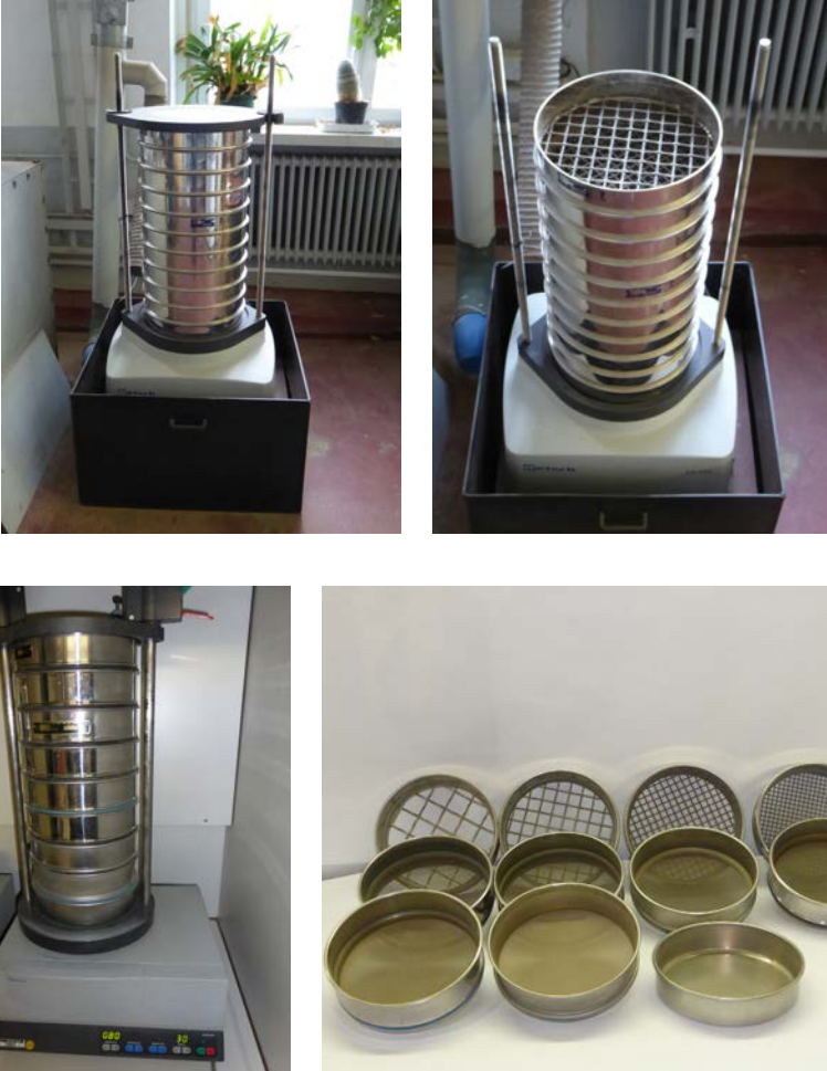
FIG. 5.4. Sieving equipment (grid size 2–32 mm).
