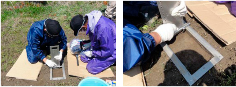
FIG. 8.14. Scraper plate for collection of soil samples for depth profiles of nuclides. (Courtesy of Yu. Onda, Tsukuba University, Japan.)
