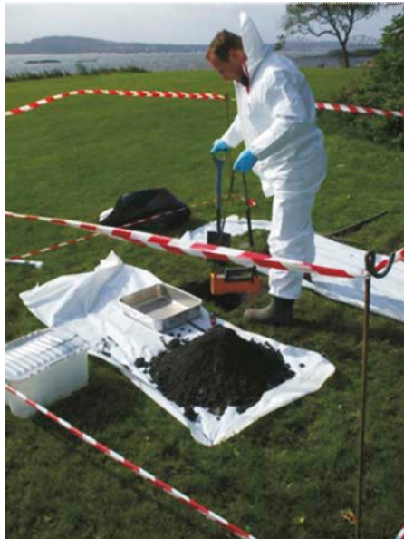
FIG. 8.49. Site excavation for the sampling and recovery of ^{226}\text{Ra} contaminated soil and artefacts on the Dalgety Bay headland.
